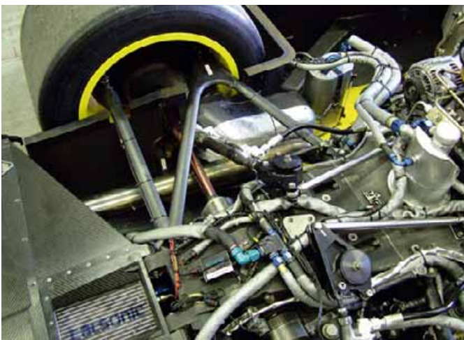
RFH car was equipped for swap to standard springs and dampers for the race
