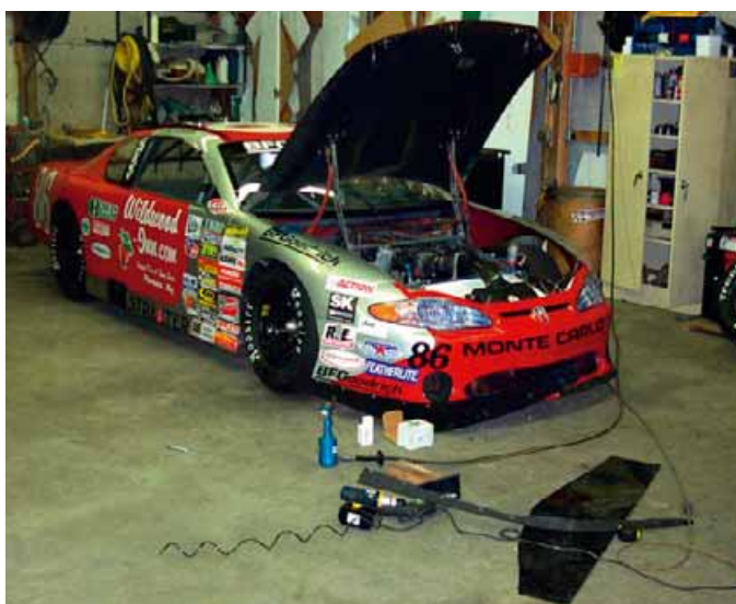
Composite bodywork from Five Star is simple, durable and, at $4000 for a complete 'shell with windows, affordable too
