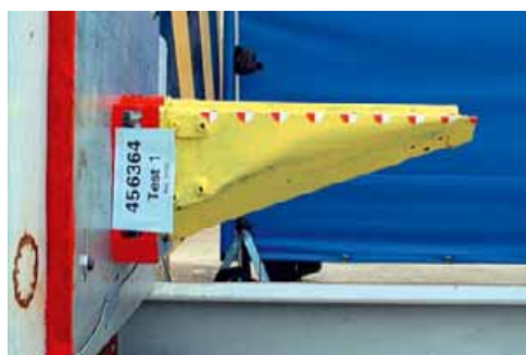
MIRA's F1 buck was constructed to undertake development work with the FIA on cockpit regulation changes
