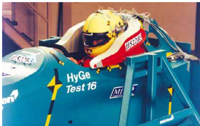
MIRA's F1 buck was constructed to undertake development work with the FIA on cockpit regulation changes
