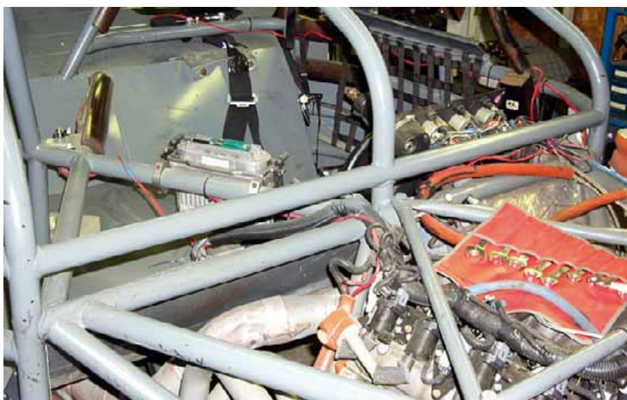
358ci V8 engines are all approved, production-based iron blocks with specified stock heads and intakes and a standard Holley four-barrel carb
