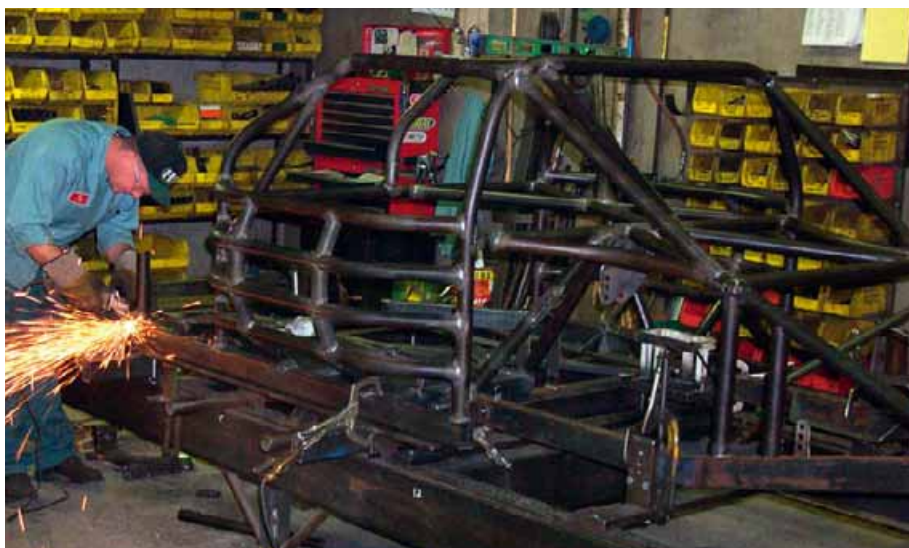
All GT-A cars use a similar spec steel tube frame stock car chassis constructed by Howe Racing Enterprises
