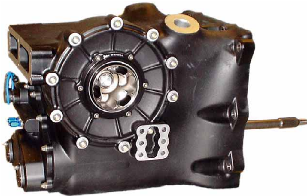
Xtrac's new longitudinal 429 'box uses the cluster from the 229 turned through 90 degrees
