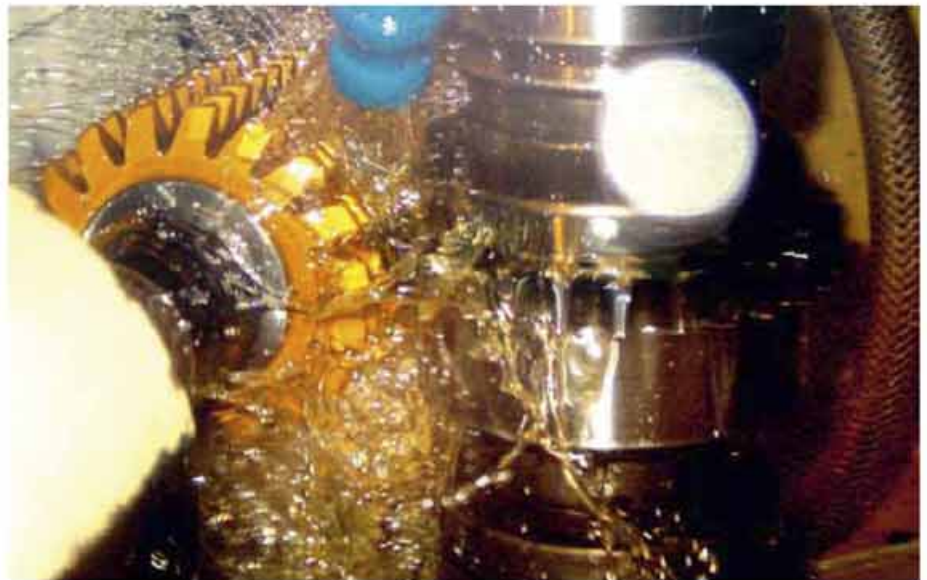
Machining gears at the Hewland factory in Berkshire where most of the work is bespoke manufacturing
