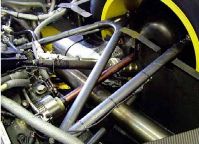
No spring and no damper are the most obvious visual differences in the system, replaced instead by a single hydraulic gas and oil filled cylinder at each corner
