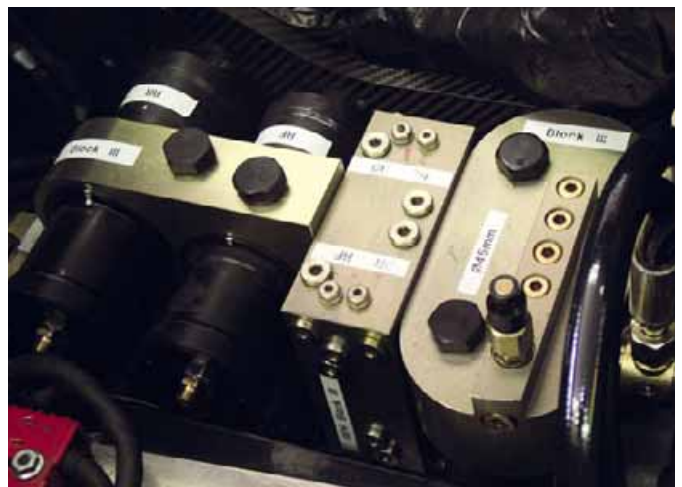
Central block allows individual spring/damper control of each chassis mode
