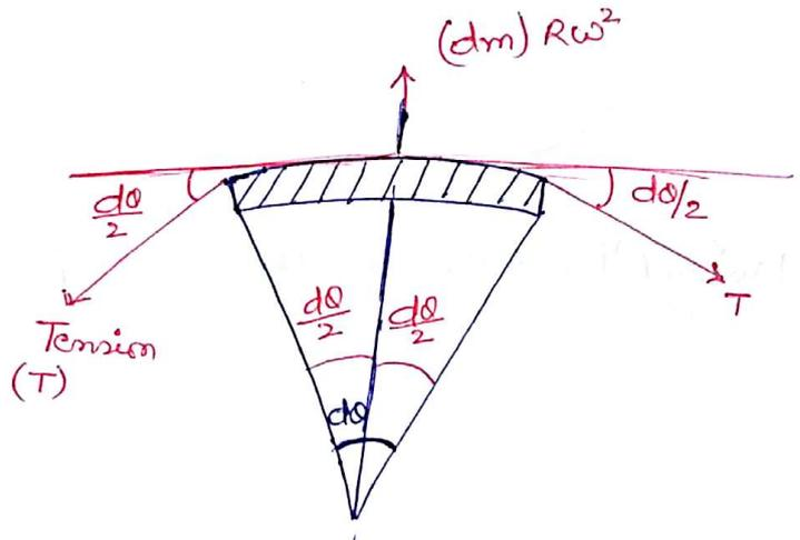
At high speed :- Disc shaped flywheel
