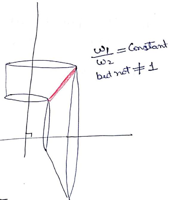
**Mitre Gear** → Use to Couple the Governor with the engine
