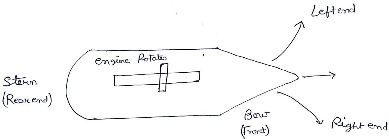
1) View from Bow (Front): engine Rotates Anti clockwise
