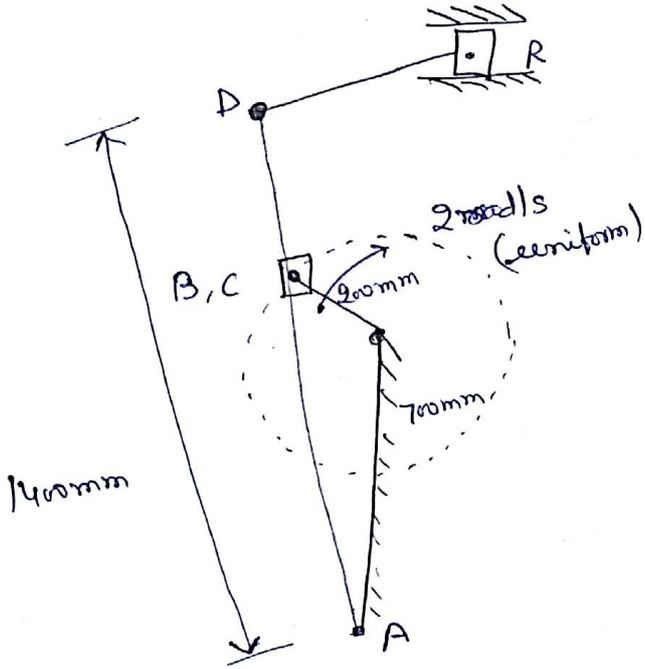
find the Avg. Velocity of Slotted Base, when vel. of RAM is Max.
