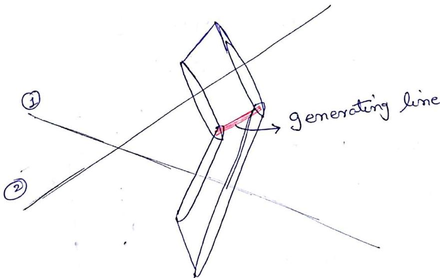
→ Pure Rolling motion, can be transmitted b/w two conical surfaces in contact.
