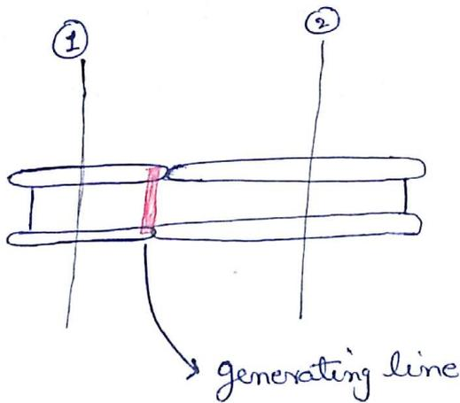
Pure Rolling motion can be Transmitted b/w two cylindrical Surface in Contact.
