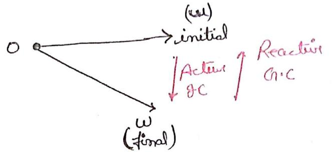
Gyroscopic Effect on ship during Pitching: Engine Rotates Clockwise.
