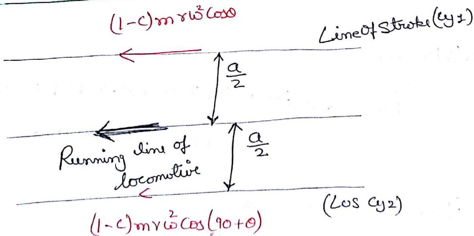
$$\begin{aligned} \text{Tractive force} &= (1-c) m r \omega^2 \sin \theta + (1-c) m r \omega^2 \cos(90+\theta) \\ &= (1-c) m r \omega^2 (\cos \theta - \sin \theta) \end{aligned}$$
