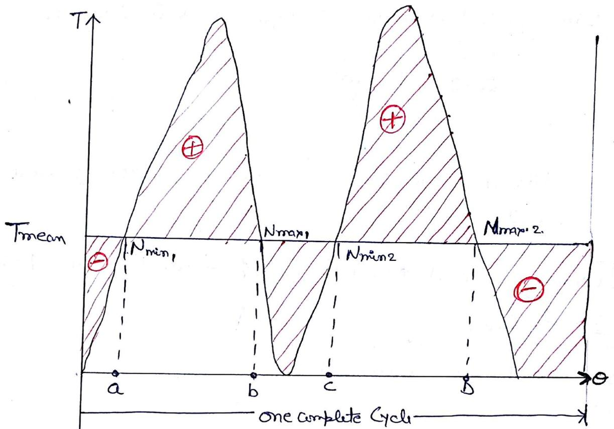
$$C_E = \frac{(E_{\max} - E_{\min})}{W_{\text{cycle}}}$$
