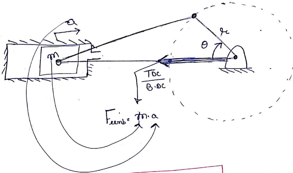
$$F_{\text{unbalanced}} = m r \omega^2 \left\{ \cos \theta + \frac{\cos 2\theta}{n} \right\}$$
