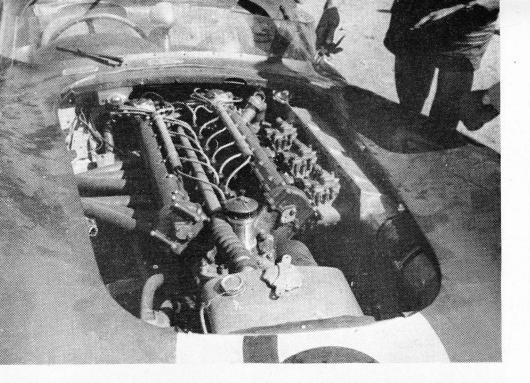
WINNING POWER-UNIT. The wellproved six-cylinder engine of the Aston-Martin DBR1.
