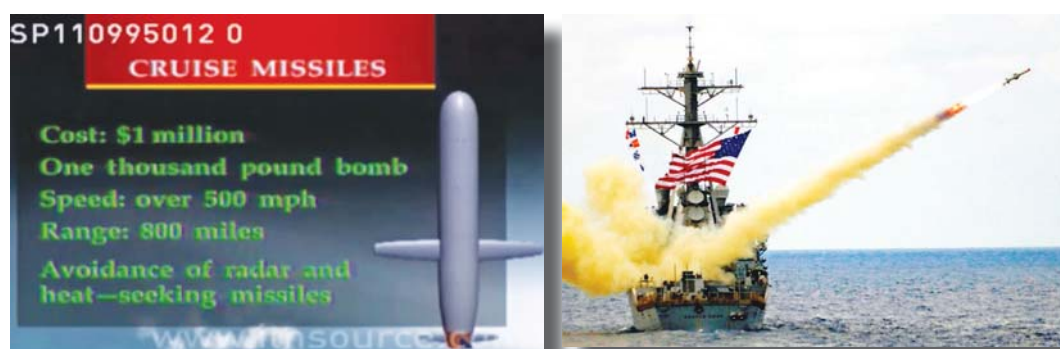
Picture 37. “Tomahawk” missile. In the picture: missile specification and the launching of the missile from the US Navy ship
