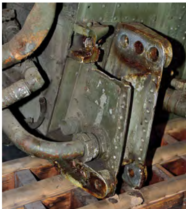
ABOVE: A close-up view of the damage to the Spitfire's port upper spar boom stub, which will be repaired. This is believed to have been sustained while X4590 was a travelling static exhibit from the 1950s to the 1970s.
