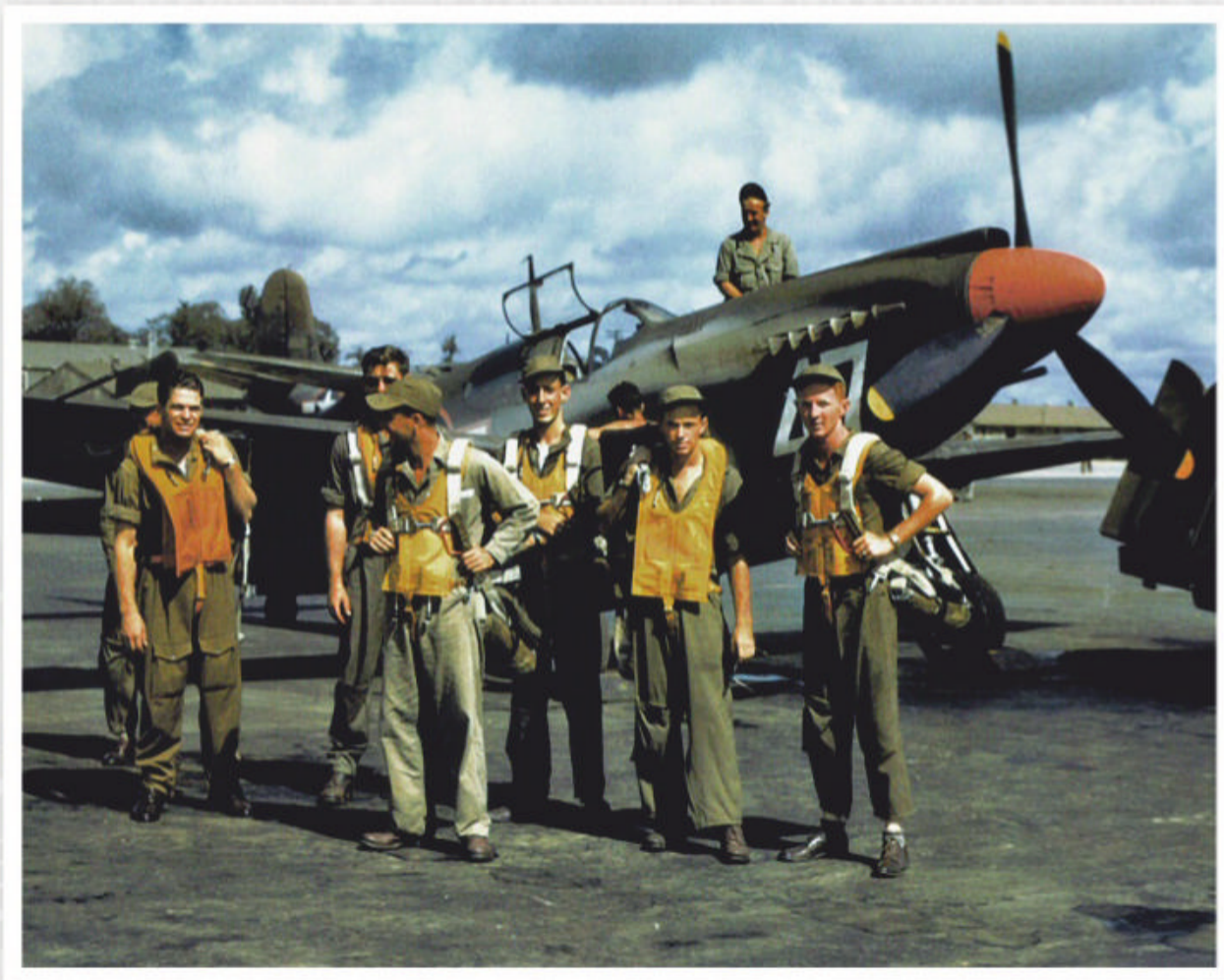
ABOVE: An A-36A refuelling while aircrew pose for the photographer. The aircraft wears the Type Three national marking with red borders introduced in June 1943. The spinner is red, indicating an aircraft bound for the Mediterranean, while the number on the nose (the last two digits of the serial) tended to be applied as an identification feature in the US. [All images via Matt Willis]
