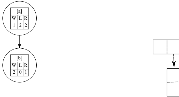
(a) Task graph with emphasis on properties, W is weight, L is level, R is resource demand (b) Task graph with emphasis on representation
