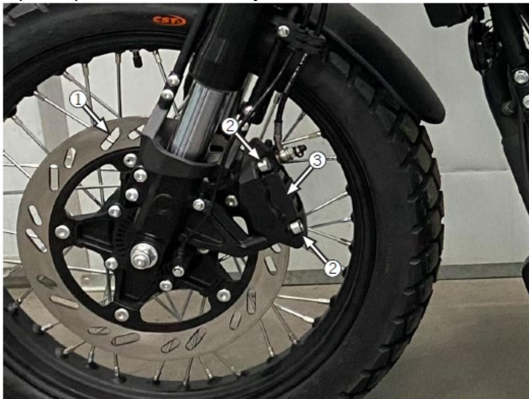
1 Front brake disc, 2 Brake caliper bolts, 3 Front brake caliper
