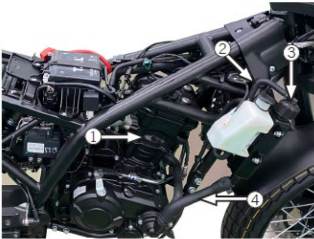
1 Engine, 2 Short circle hose/ water pipe, 3 Water tank cover, 4 Water outlet hose/ water pipe, 5 Radiator, 6 Water inlet pipe, 7 Thermostat, 8 Temperature sensor
