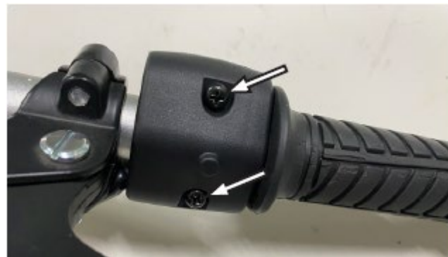
6. Remove the handlebar clip fixing bolt.
