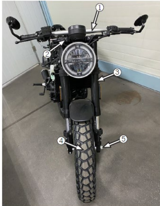
1 Control subassembly, 2 Upper connecting plate, 3 Front fork assembly, 4 Front wheel components, 5 Front axle
