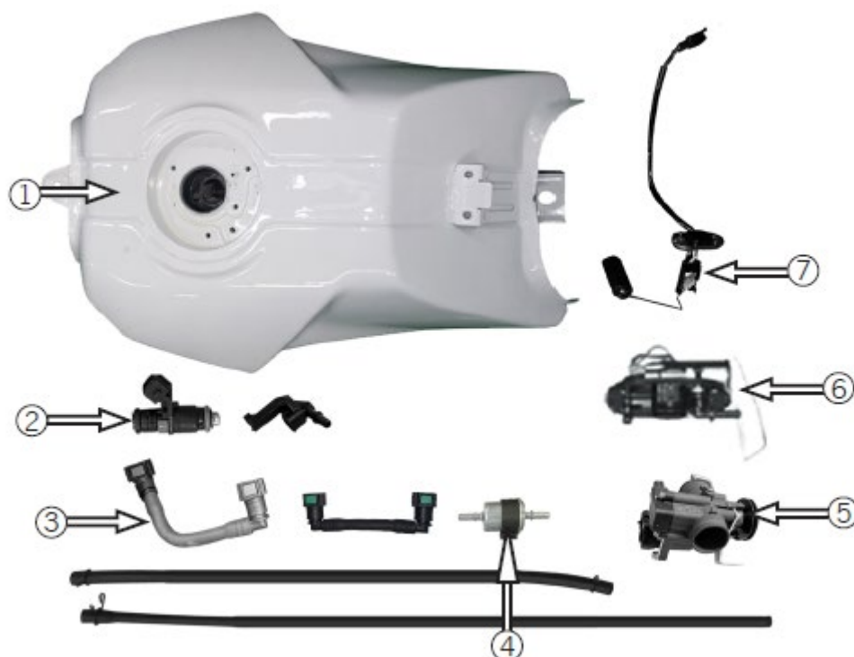
1 Fuel tank, 2 Fuel injector, 3 High pressure pipe, 4 Air cleaner, 5 Valve body, 6 Fuel pump, 7 Fuel sensor
