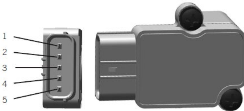
1 Inlet pressure signal, 2 5V reference voltage, 3 5V reference voltage grounding, 4 Throttle plate position signal, 5 Inlet temperature signal
