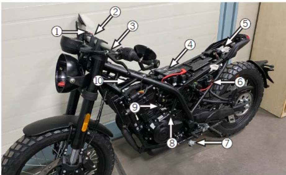
1 Engine stop, 2 Starting switch, 3 Clutch switch, 4 Battery, 5 ECU, 6 Starting relay, 7 Side bracket switch, 8 Gear switch, 9 Starting motor, 10 Cable harness
