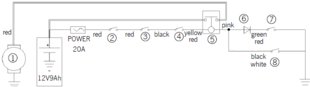
1 Starting motor, 2 Ignition switch, 3 Engine stop, 4 Electric starting switch, 5 Starting relay, 6 Isolation diode, 7 Neutral switch, 8 Clutch switch
