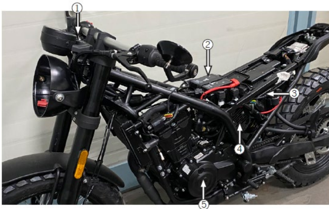
1 Ignition switch, 2 Main electrical harness, 3 Battery, 4 Voltage regulating rectifier, 5 Magneto
