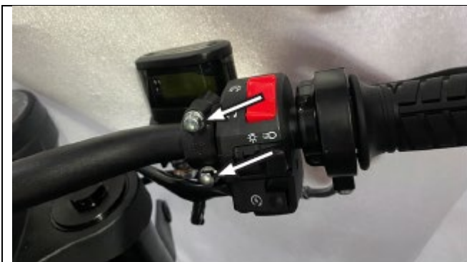
3. Remove the right combined switch screw.
