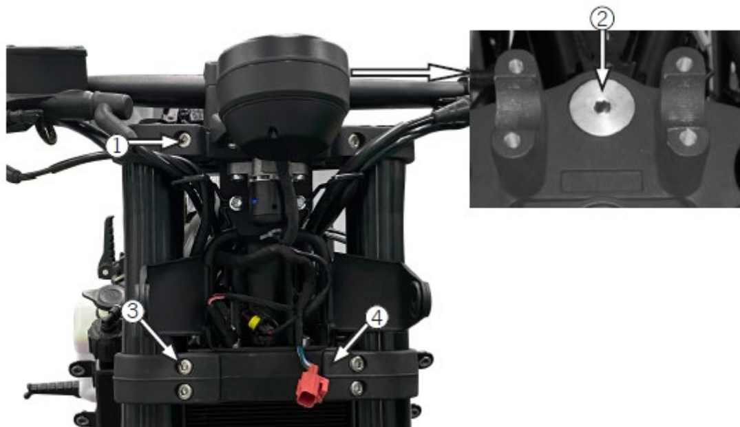
1 Upper damping bolt, 2 Steering column locking bolt, 3 Lower damping bolt, 4 Steering column combination
