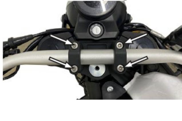
6. Remove the handlebar clip fixing bolt.
