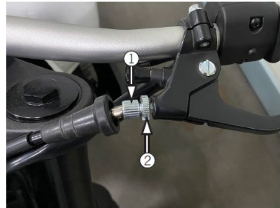
1 Adjust nut, 2 Lock nut
