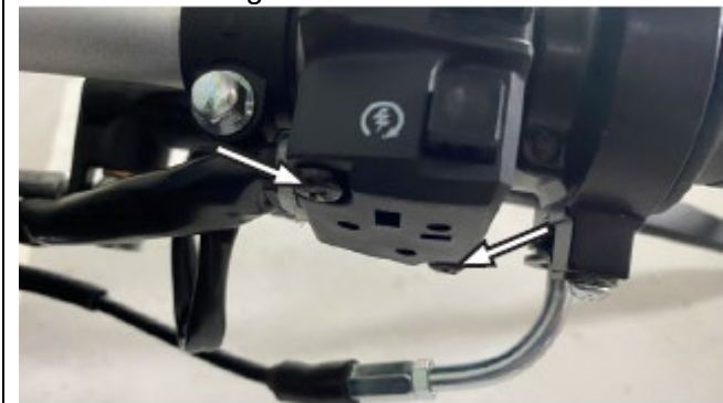
4. Remove the fixing screw of throttle cable wire seat, and remove the fixing screw fasten throttle cap screws.
