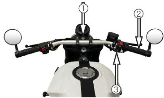
1 Turn the key clockwise, 2 Fully open the throttle handle, 3 Press the electric start button
