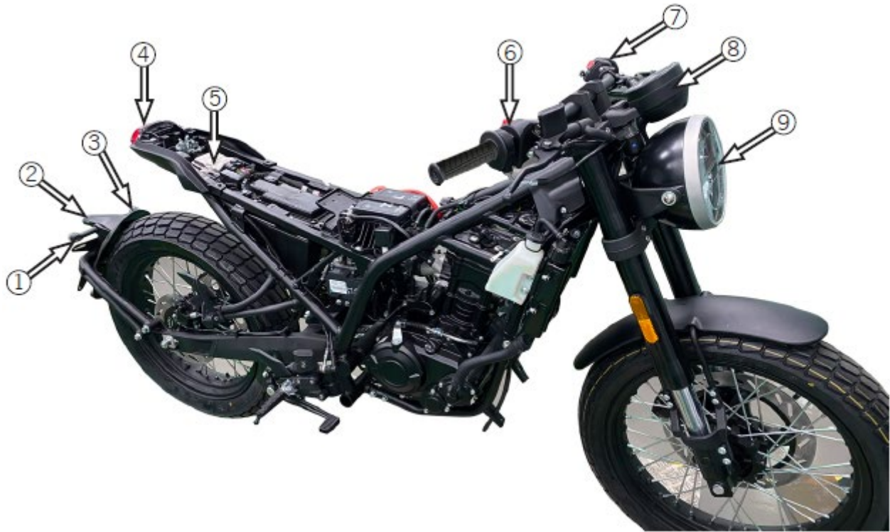
1 Rear right direction indicator lamp, 2 Rear license plate lamp, 3 Rear left direction indicator lamp, 4 Combination tail lamp, 5 ECU, 6 Right combination switch, 7 Left combination switch, 8 Meter, 9 Headlamps
