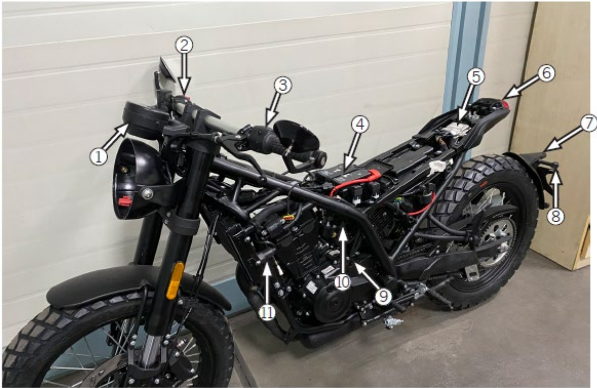
1 Instrument, 2 Right combination switch, 3 Left combination switch, 4 Battery, 5 ECU, 6 Combination tail lamp, 7 Rear registration plate lamp, 8 Rear left direction indicator lamp, 9 Sensor, 10 Three in one sensor, 11 Water temperature sensor
