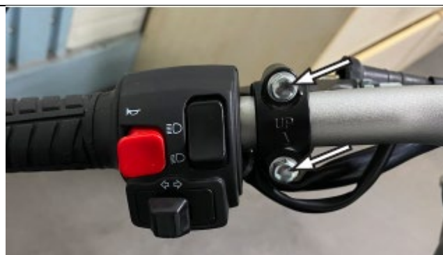
7. Remove the left combined switch screw.
