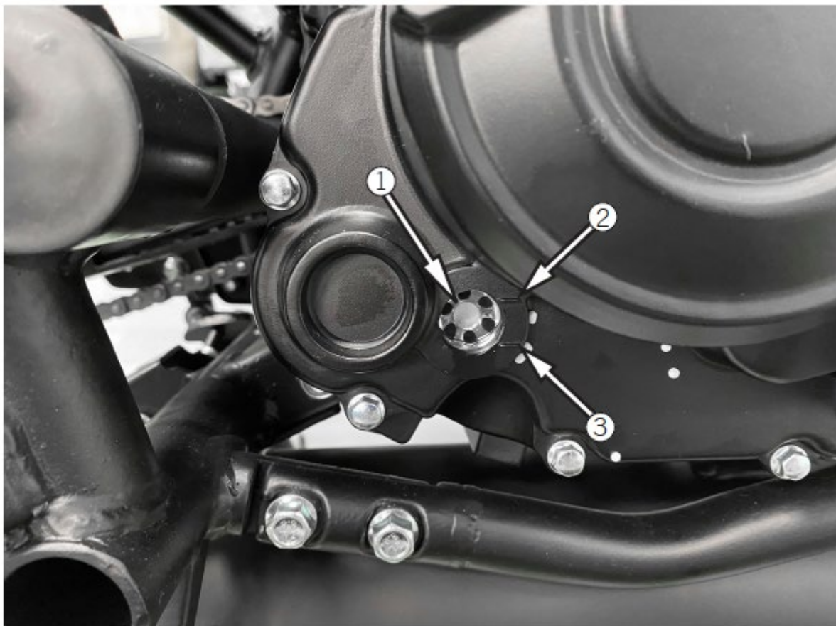
1 Engine oil sight window, 2 Engine oil upper limit line, 3 Engine oil lower limit line
