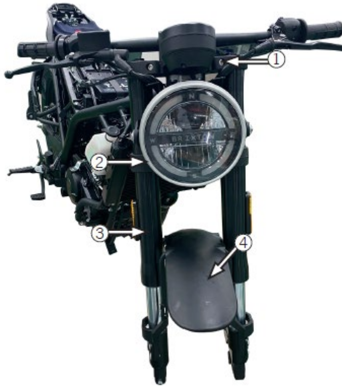
1 Upper shock absorber bolt, 2 Lower shock absorber bolt, 3 Front shock absorber, 4 Front fender
