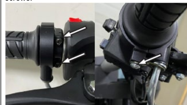
4. Remove the fixing screw of throttle cable wire seat, and remove the fixing screw fasten throttle cap screws.
