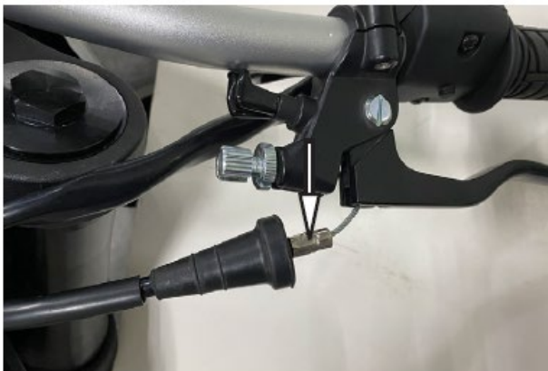
Remove the clutch operating line
