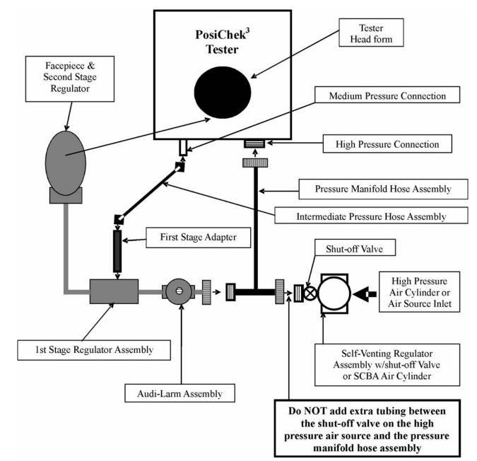
MSA Air Mask Connection to the Posichek<sup>3</sup> Tester Schematic
