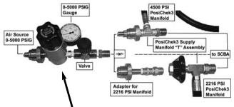
Self-Venting High-Pressure (0 to 5000 psig) Regulator and Shut-Off Valve Assembly Biosystems (P/N 35-0470)
