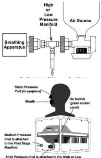
High Pressure Inlet is attached to the High or Low Pressure Manifold (as appropiate for the BA)
