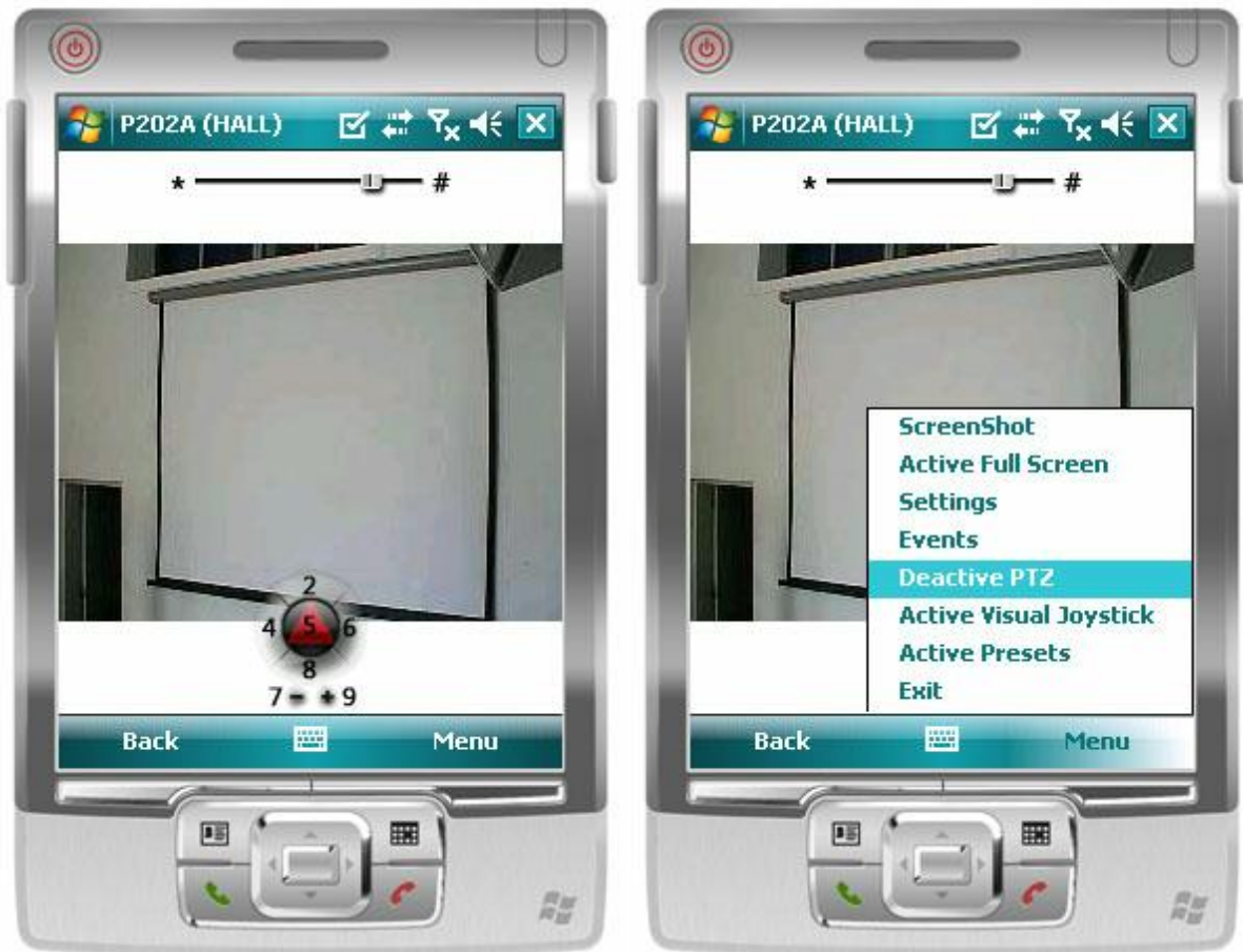
(Fig. 42 and 43) Control and deactivation of PTZ
