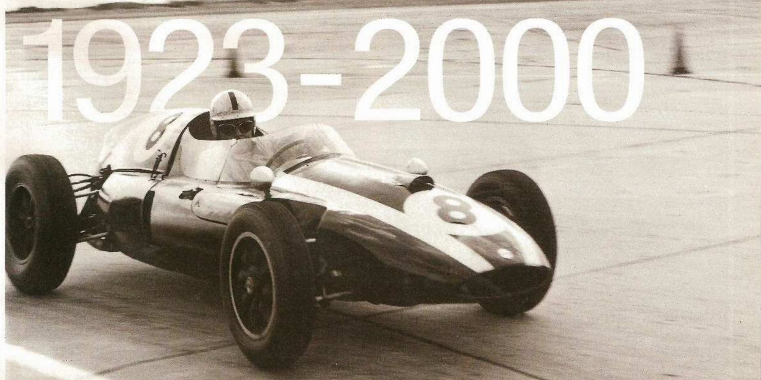
Jack Brabham races a Cooper T51 in the 1959 US Grand Prix at Sebring. The rear-engined model revolutionised race car design and secured driver and constructor titles in '59 and '60
