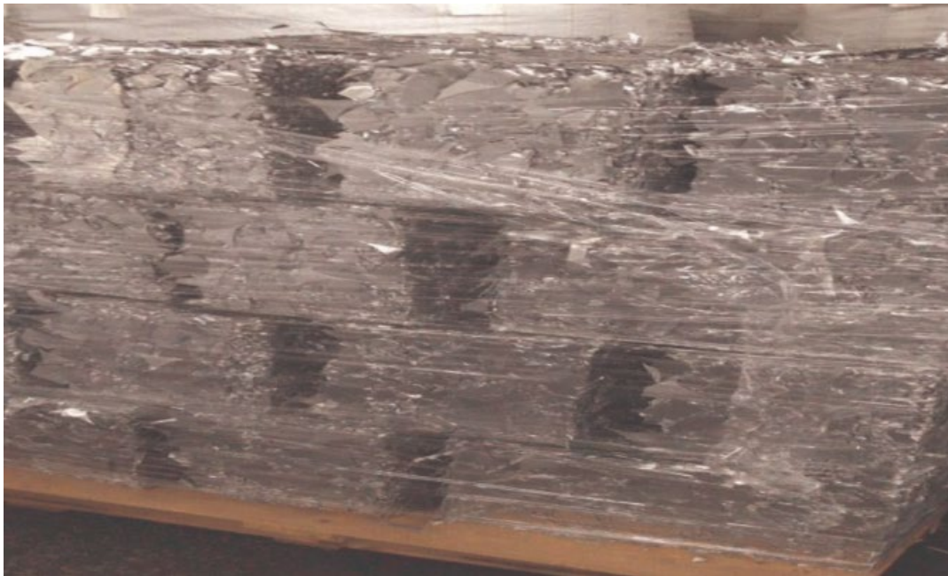
Figure D.8 Compaction package of small material - from mixed new processing remnant materials and geometric waste materials
