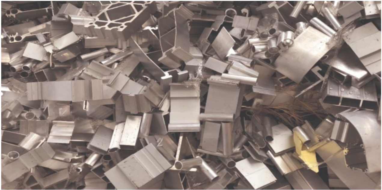
Figure D.1 Bulk small material - from mixed new processing remnant materials and geometric waste materials
