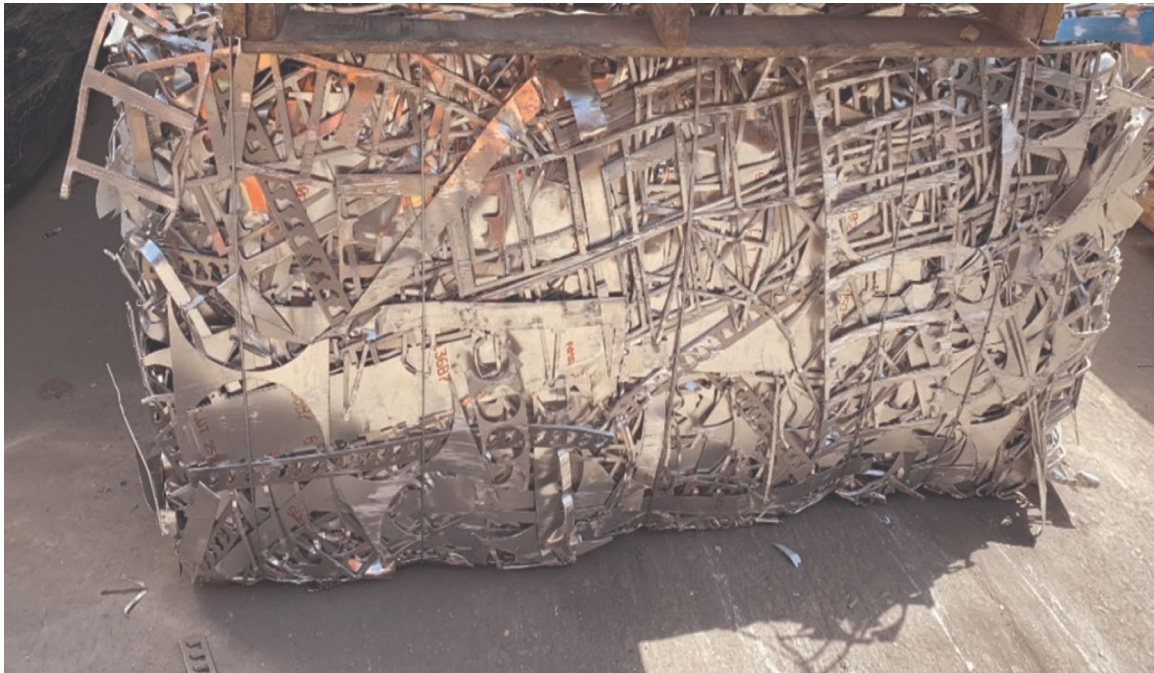
Figure C.4 Easily disassembled package of small material - from mixed new processing remnant materials and geometric waste materials
