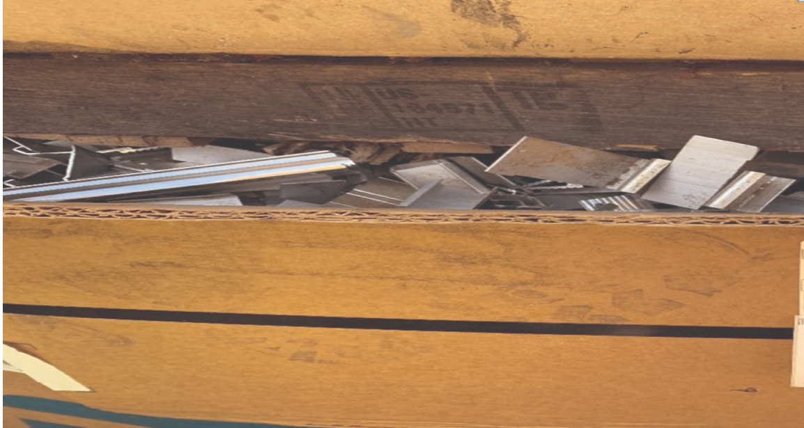
Figure C.1 Bulk small material - from mixed new processing remnant materials and geometric waste materials
