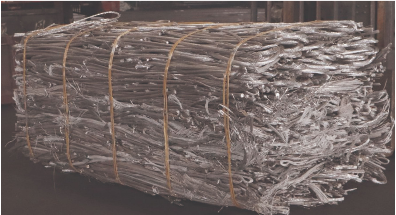
Figure B.14 Easily disassembled package of large material (light) - from aluminum wire (cable) of the same brand
