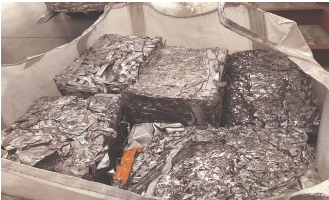
Figure B.15 Compaction block of small material - from new processing remnant material and geometric waste material of the same brand
