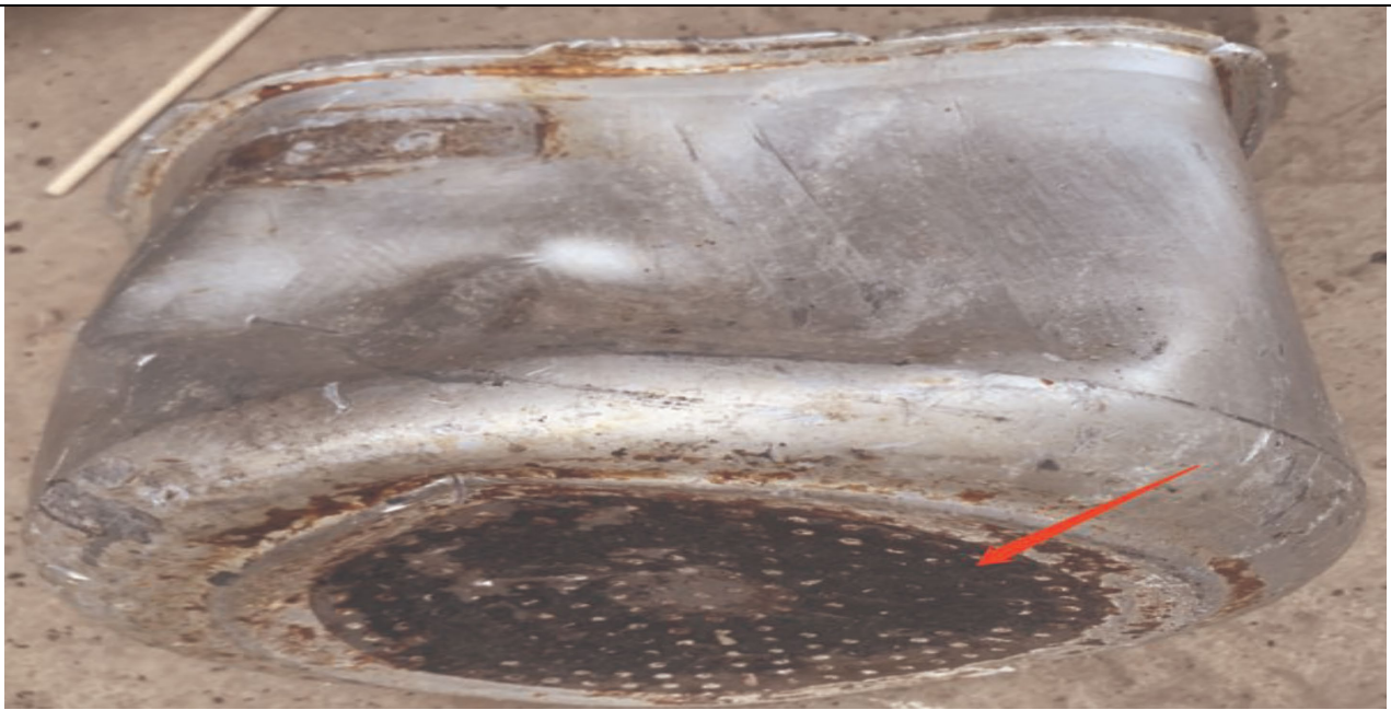
Figure A.9 Iron inlay in aluminum pot
