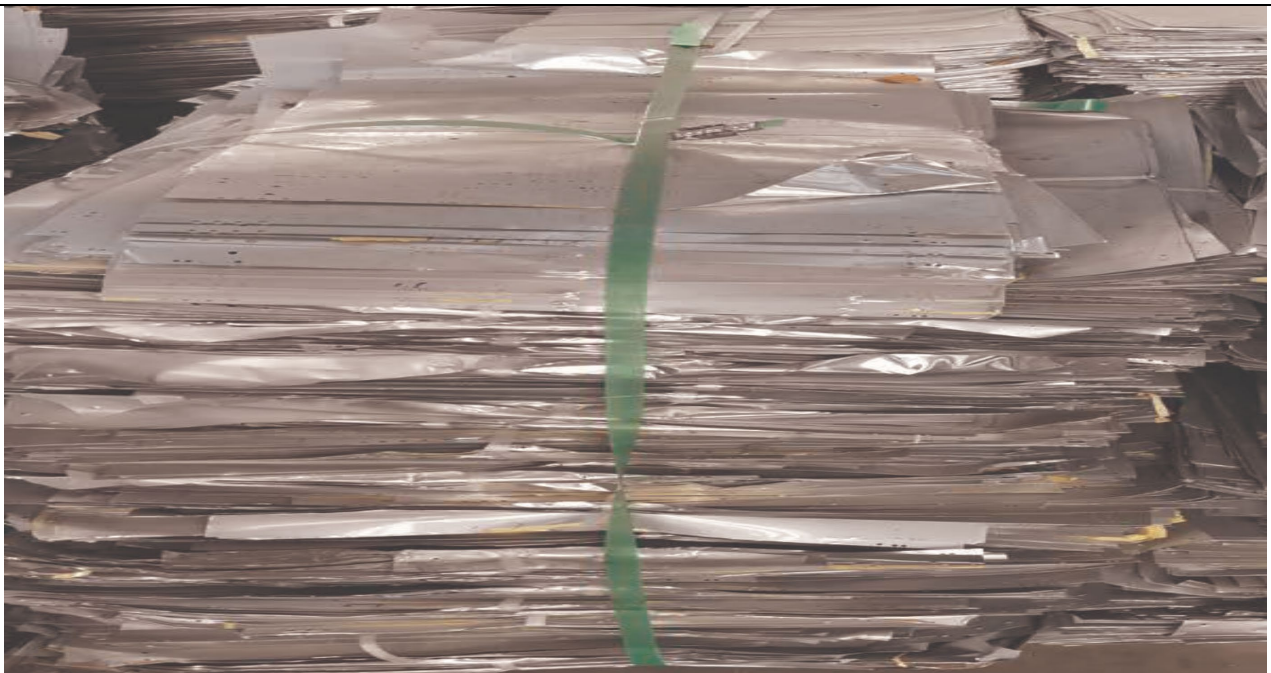
Figure B.5 Bulk small material - from the new clean printing plate base
