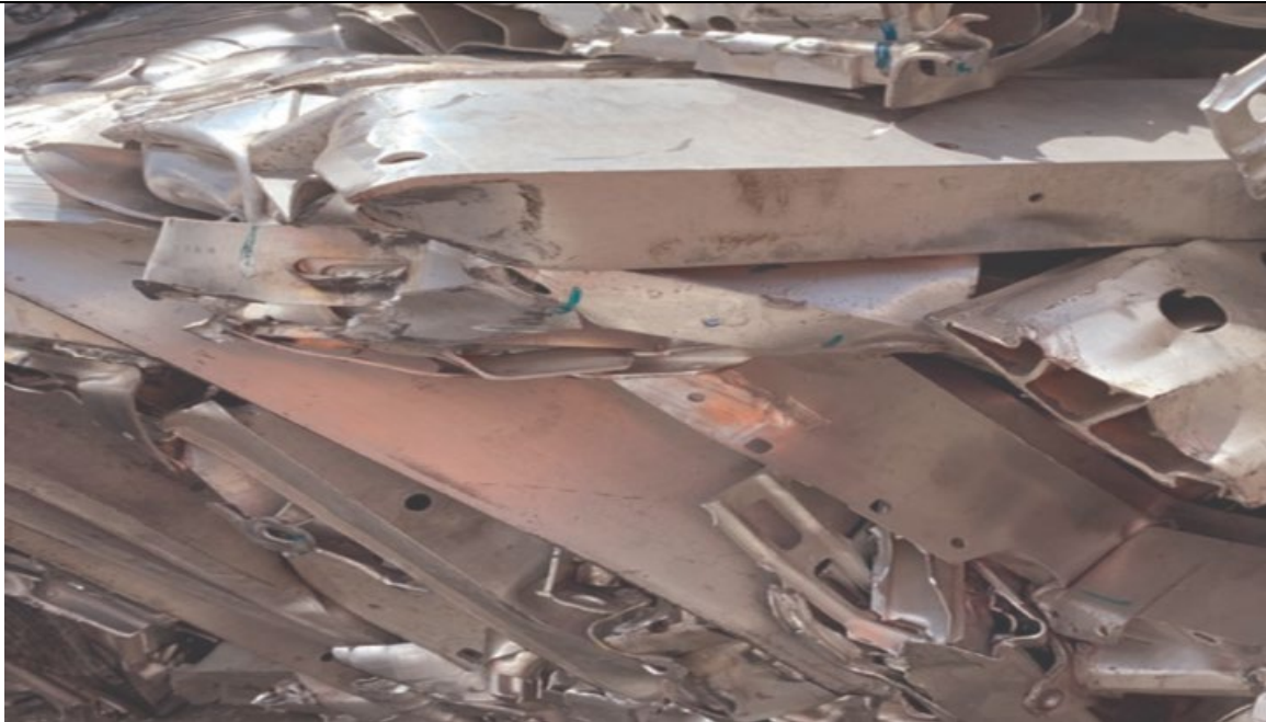
Figure D.5 Easily disassembled package of large material (heavy) - from mixed old extruded material
