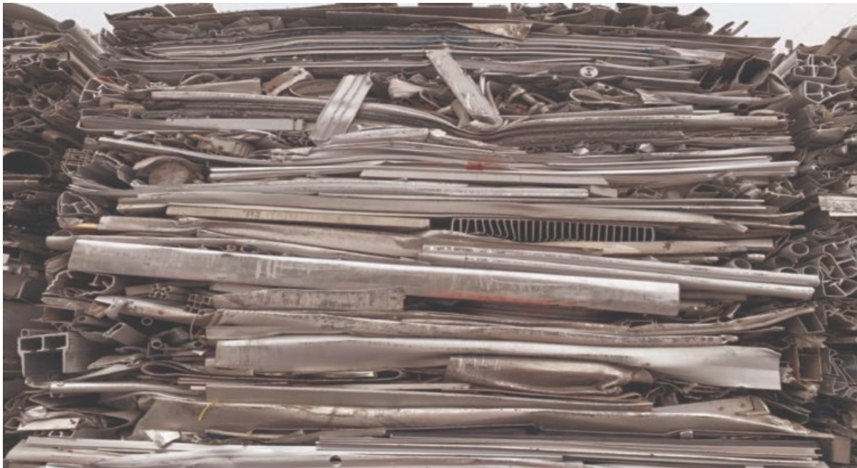
Figure D.6 Easily disassembled package of large material (heavy) - from mixed old aluminum
