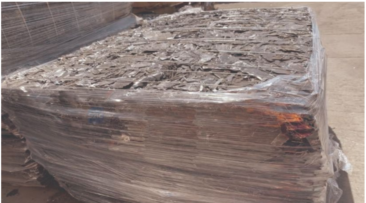
Figure D.2 Bulk small material - from the clean printing plate base
