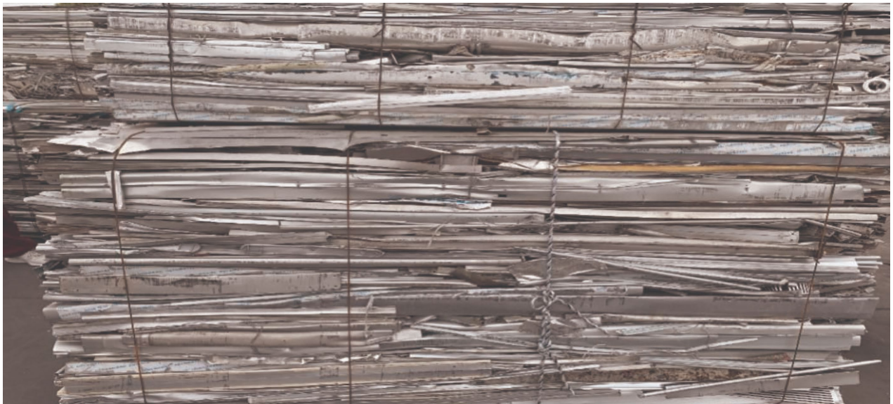
Figure C.2 Bulk large material (light) - from extruded material "10/10"
