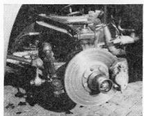
SERVO-ASSISTED Dunlop disc brakes are fitted all round.
