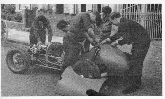
is necessary because single triangulated tubular radius arms are used, located by ball joints well forward on the chassis. Lateral location is by a slide on the differential housing, and the rear wheels have a negative camber of 2 degrees.
