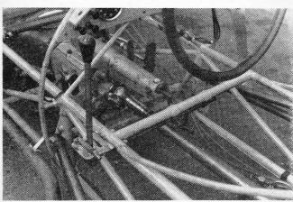
FROM ABINGDON (above) comes the gearbox, being of M.G. TC type, with remote control to the lever on the left
