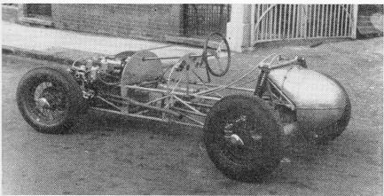
LAID BARE: (Above) Everything fits neatly into the frame of the Lister, which is made of 1 in. and  $\frac{3}{4}$  in. steel tubing, and weighs only 32 lb. bare. Note the semi-spherical fuel tank in the tail.
