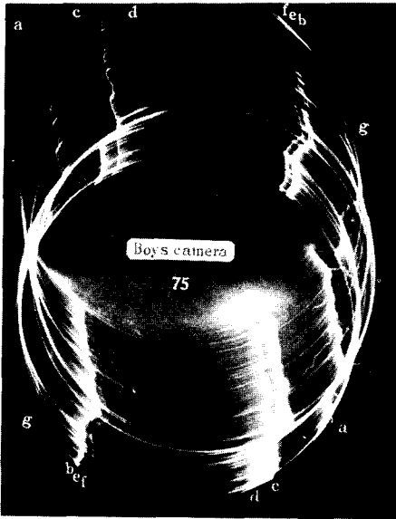
Fig. 9-14. Photograph of a lightning flash taken with a "Boys" camera. [From Schonland, Malan, and Collens, Proc. Roy. Soc. London , Vol. 152 (1935).]
