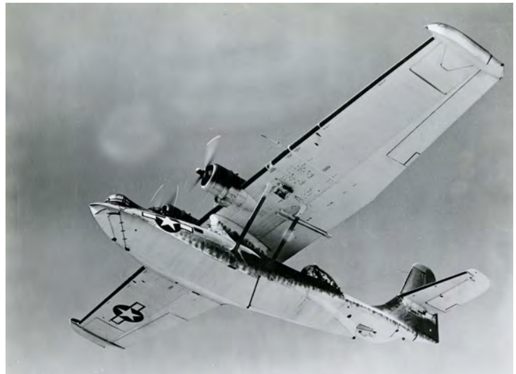
One of the most distinctive and best-loved shapes in aviation, the Consolidated Catalina. This version is a Naval Aircraft Factory-built PBN-1 Nomad, a variant derived from the PBV-5 but featuring a sharper bow, extended aft hull step and redesigned taller tail.
