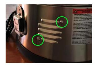
On older units, these may have come from the factory tightened a little too snug. Locate the screws by the vent at the bottom of the unit, generally where the sound is coming from, and loosen them 1/4 - 1/2 a turn.
