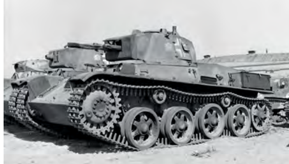
The 38M Toldi light tank, the licence version of the Swedish L-60 tank was the platform of the 40M Nimród Sp. AA-AT vehicle. FORTEPAN
