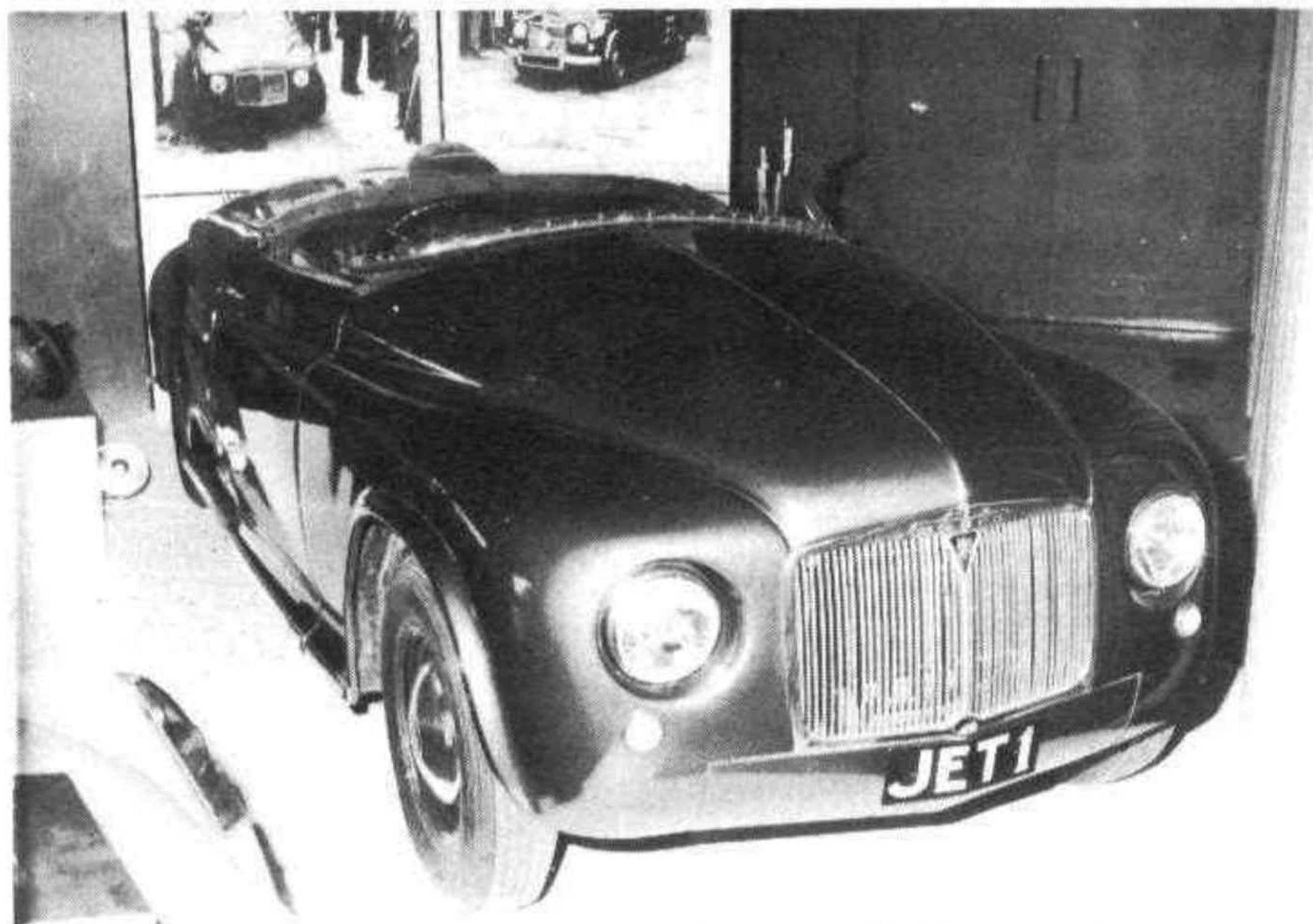
The first Rover turbine car, which covered the two-way kilometre at 151.965 m.p.h. and the two-way mile at 151.196 m.p.h., World's Records.
