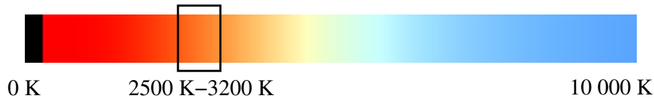
Figure 7.10: Black-body radiator colors from 0^\circ K to 10000^\circ K . Fire particles belong to temperature values from 2500^\circ K to 3200^\circ K .
