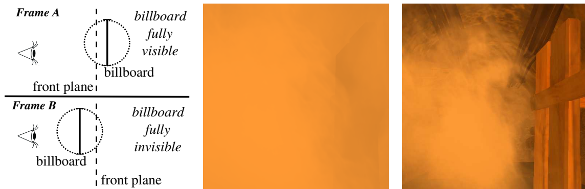
Figure 7.2: Billboard popping artifact. Where the billboard gets to the other side of the front clipping plane, the transparency is discontinuous in time (the figure shows two adjacent frames in an animation).
