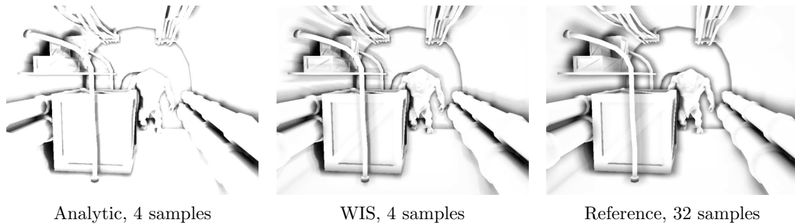
Figure 4.10: Effects of the proposed weighted importance sampling (WIS). Note that the image rendered with weighted importance sampling from 4 samples is much closer to the reference image generated from 32 samples.
