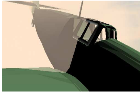
Figure 8.3: Problems caused by objects in a volume rendered as billboards. Where the billboard plane intersects the object, transparency becomes discontinuous.
