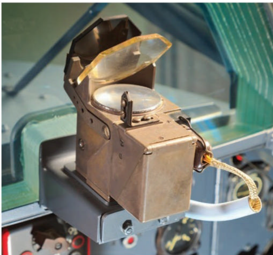
The common Revi 16/B, reflector, noncomputing gun sight was used.
