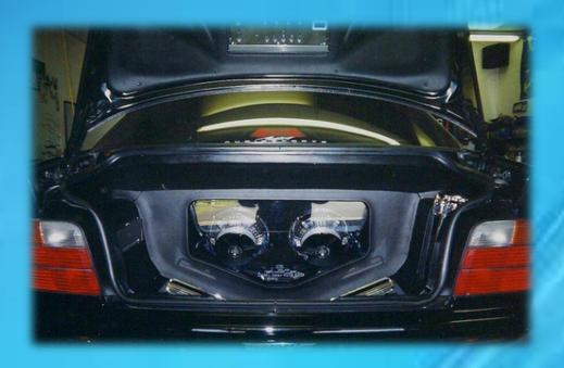
This BMW was built for one of the owners the store He wanted to turn heads. especially when the sound system was playing. Master audio & security then installed a system worthy of being in a magazine. Custom door panels and a customized trunk with a Plexiglas's view of the subwoofers. The equalizer was installed under the trunk lid. custom LED lighting. All the custom panels were then wrapped in ultra leather. This BMW has won many trophies.
