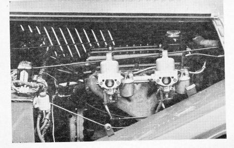
NINETY B.H.P. is delivered by the 2-litre TR2 engine fitted in the car tested. The large-bore twin SU carburetters are standard.
