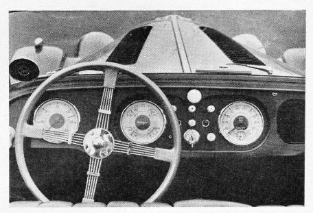
OFFICE: Large, easy-to-read instruments are provided on the well-planned facia panel of both left-hand and right-hand drive models.
