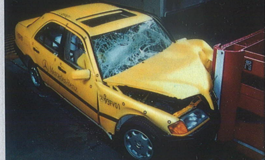
The most common type of accident: the offset crash. It has been a part of our test programme since the 1970's.
