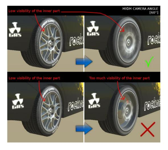
The angle between the camera and the wheels depends on the orientation of the single wheel (left or right), so all the wheels on left side must have a localScale.x less than zero (the opposite value of the corresponding right wheel). Check the example scene to see how the wheels are positioned. It's easy to customize the way S.W.E. gets informations about the wheel orientation: just change the lines 362 and 390 of the SpinEffect.cs script.
