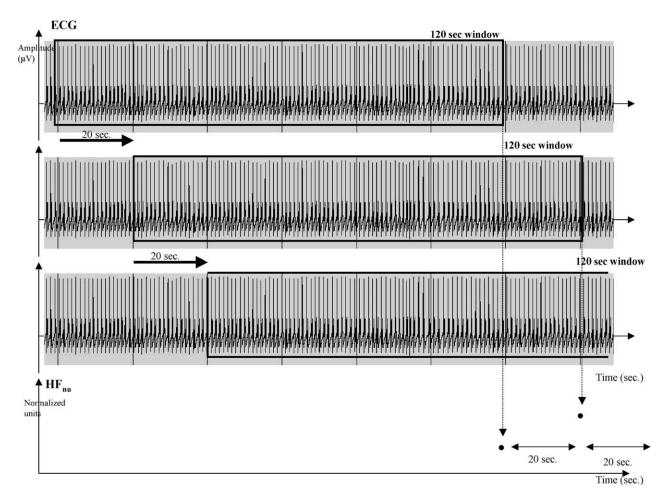
Fig. 1. The RRI power spectrum components,  $LF_{nu}$  and  $HF_{nu}$ , were computed from the ECG on a 120 s window. This 120 s window was then shifted ahead by 20 s. Each 120 s window corresponded to one spectral value for  $LF_{nu}$  and  $HF_{nu}$ . As a result, a spectral value was obtained each 20 s. On this figure, only  $HF_{nu}$  is represented.
