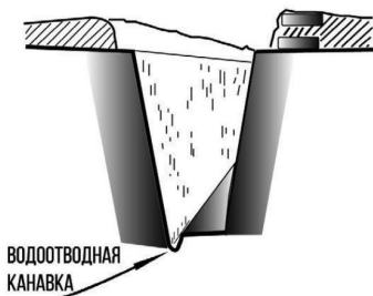
Fig. 2. Drainage ditch of trench bottom
