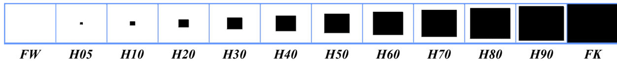
G. Targets for manifesting halation (contamination of darks with surrounding light areas).
