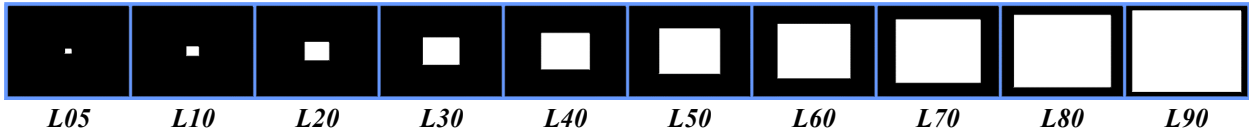
H. Targets for manifesting loading (change in luminance with size of white area).
