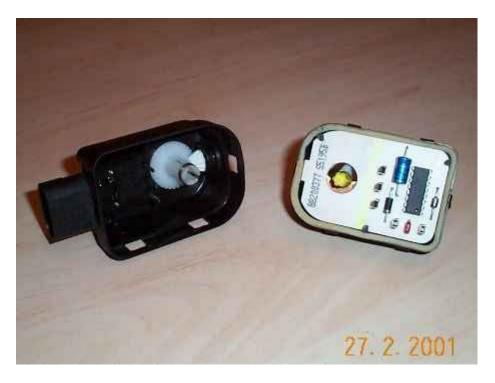
Next, prise the motor unit open. This is done by inserting a small screwdriver between the two halves and working around the groove. The part on the left contains the manual height adjuster mechanism. The part on the right is the motor and control circuits.
