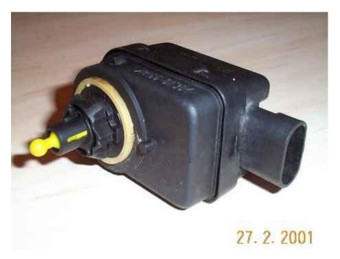
First, remove the motor from the headlamp. This is done with a quarter turn anti-clockwise of the motor unit and then sliding the yellow ball out of it's groove.
