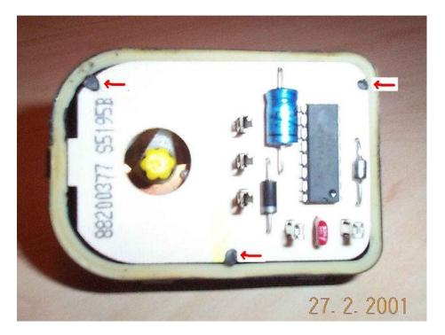
Next, use a small sharp knife to remove the head of each plastic securing rivet (arrowed) that secure the board to the assembly. This doesn't cause any problems later on.
