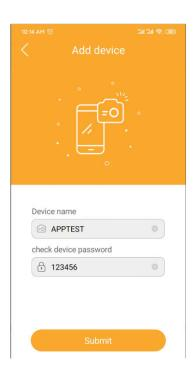
Press Submit, then camera add into app successfully, you can check the camera data and setup the camera such as APN, phone number, for example: change the mode to Camera& Video, then press" save" to save the setting.
