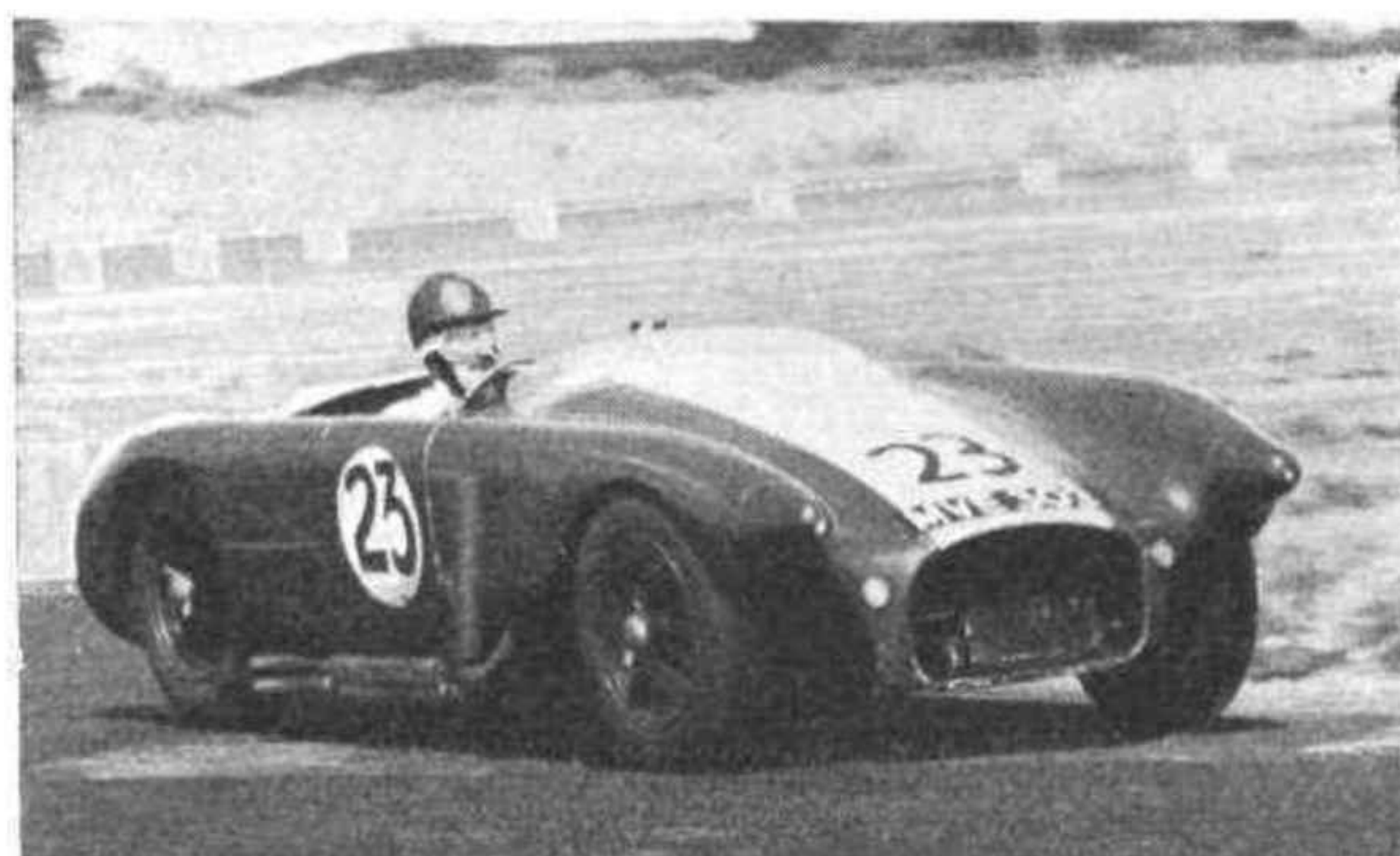
The Lister-Bristol, with frame of single tubes and a de Dion back-end, goes remarkably well in the hands of W. A. Scott-Brown, using a "normal" Bristol engine.
