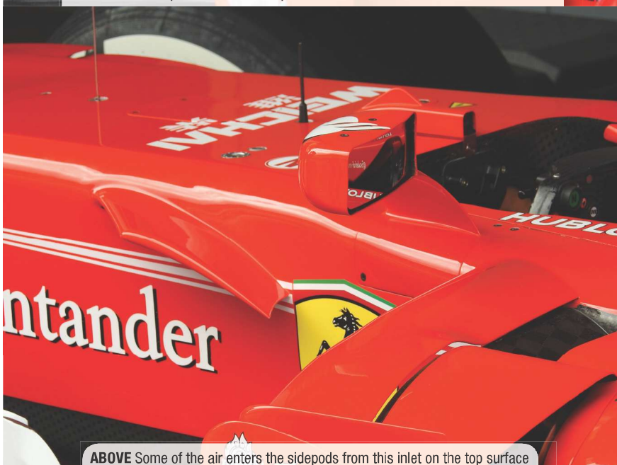
ABOVE Devices upstream of the sidepods create downwash to direct to the undercut
