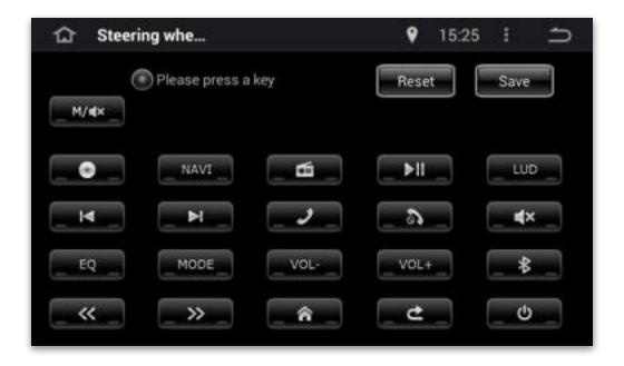
To remap a physical button you tap the function button on the Settings screen, and then press the physical button that should invoke that function. If the remap operation was successful the function button will have a colored border to indicate it has been remapped.
