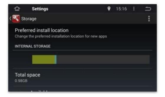
By setting the 'Preferred install location' you can decide whether applications and data are stored on the head-unit's internal or external memory. This can be useful when installing applications such as multiple GPS application that have large data files and use a lot of storage space.
