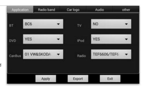
If you have purchased a generic unit you may need to change the CanBus setting to reflect the manufacturer of the vehicle it is being installed into.
