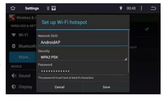
To start the HotSpot service, enable the 'Portable Wi-Fi hotspot' option.
