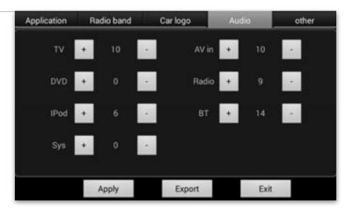
TV, and the A/V Inputs as well. It may take some time to experiment with the different levels per input, but eventually you can balance the volume across all inputs.
