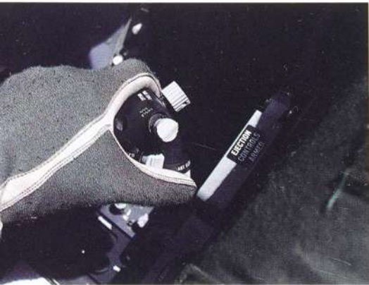
Falcon driver's left hand controls engine throttle and ten other switches. "Dog fight" button flips radar back and forth between air-to-air and air-to-mud.
