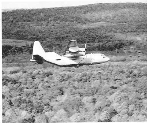
Odd antenna fins identify EC-130 Psyops Hercules, shown here in low-level pass near Harrisburg, Pennsylvania. Photo: MSgt Wayne Isett, PA ANG.
