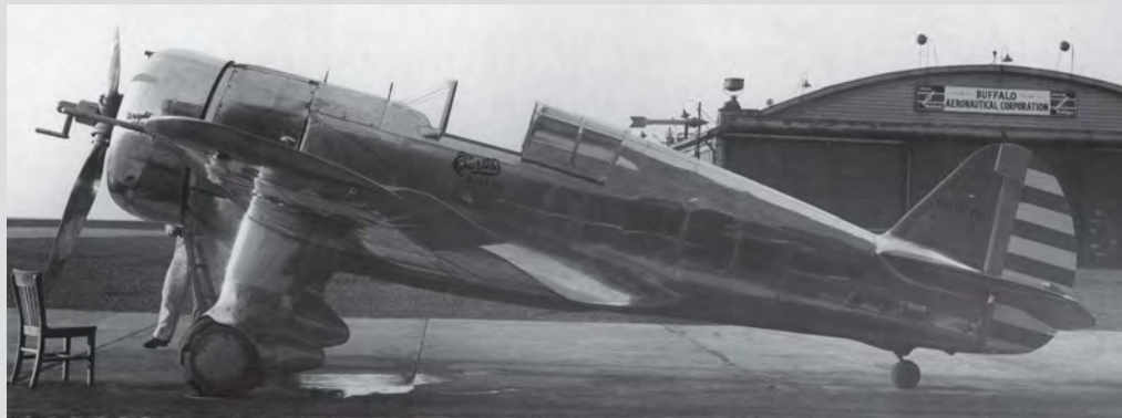
Fixed-undercarriage Hawk 75H demonstrator NR1276 was the aircraft used by Claire Chennault during his time as an advisor to the Chinese Nationalists. KEY COLLECTION
