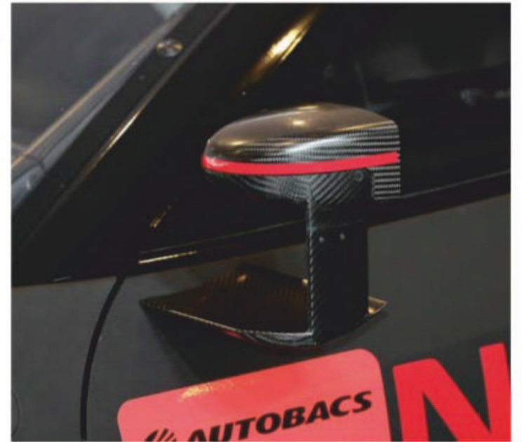
Nissan's aerodynamic mirrors follow a trend set by the DTM cars
