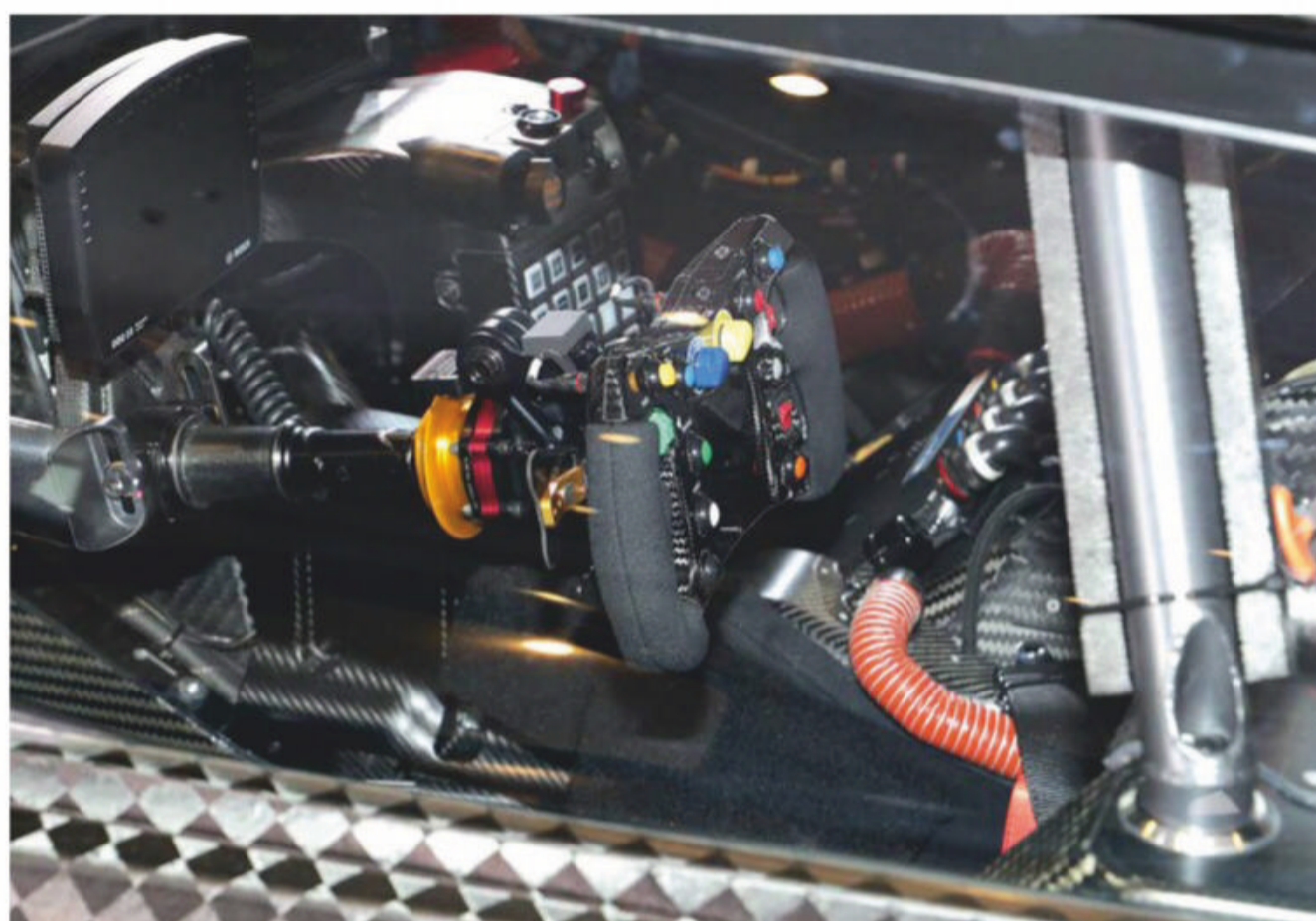
The cockpit switching and much of the electronics package, including a Bosch ECU, is now common across all Class 1 cars
