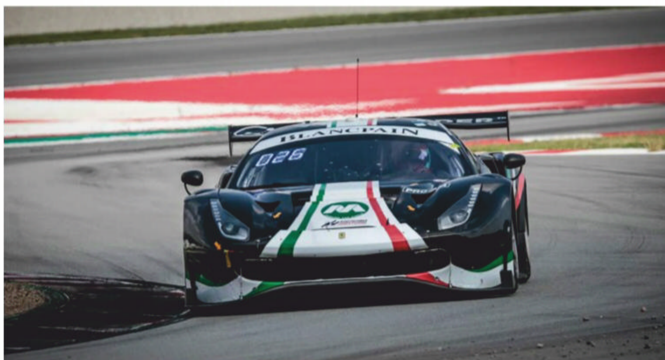
The Ferrari was the best of our cars with an almost even weight distribution, low drag and a decent amount of downforce
