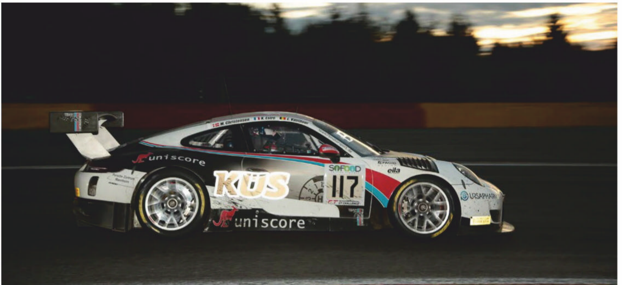
Racing Porsche GT3s allow for adjustment of 'caster' at the rear as well as at the front, but this really has much more to do with the bump steer rather than anti-lift and anti-squat
