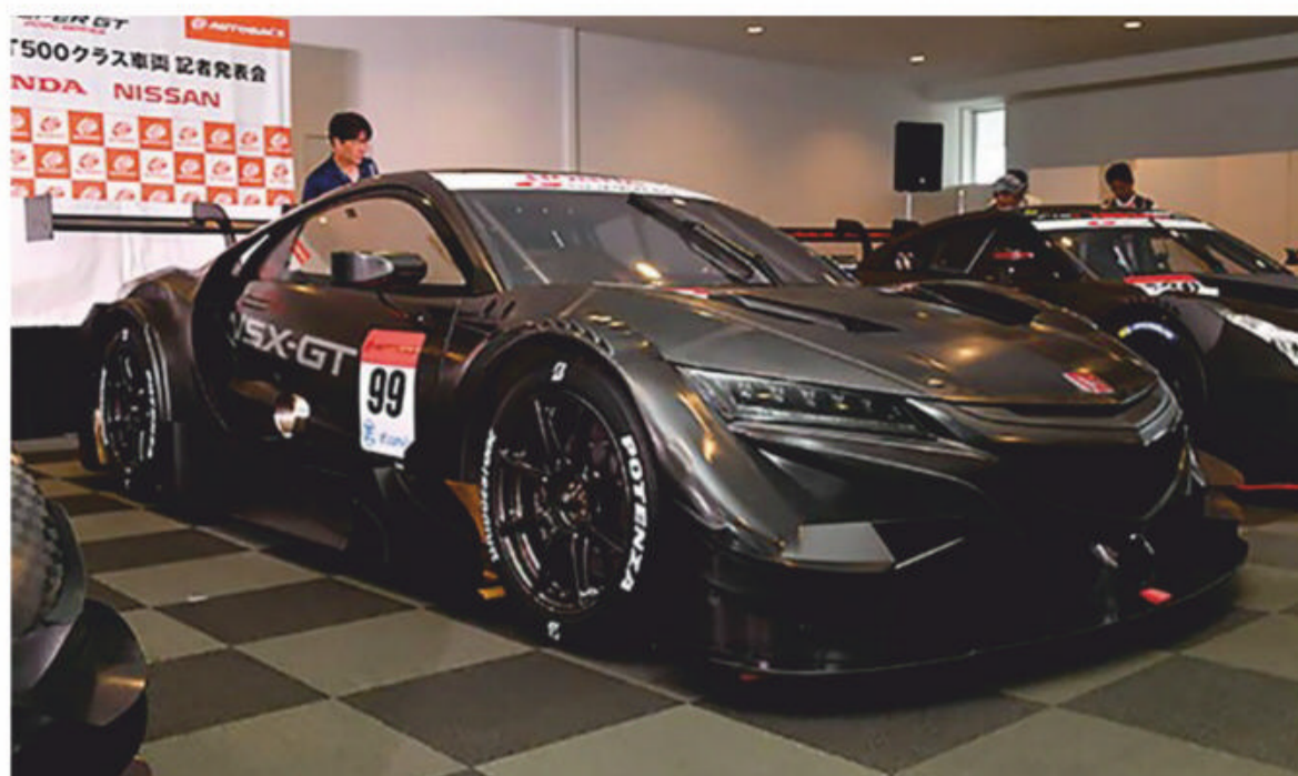
Honda's new GT500 has its engine in the front, rather than mid-mounted as it is in its 2019 Super GT racecar
