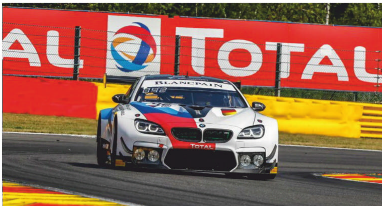
The BMW M6 GT3 should perform well in high-speed corners due to its high downforce potential and its weight distribution
