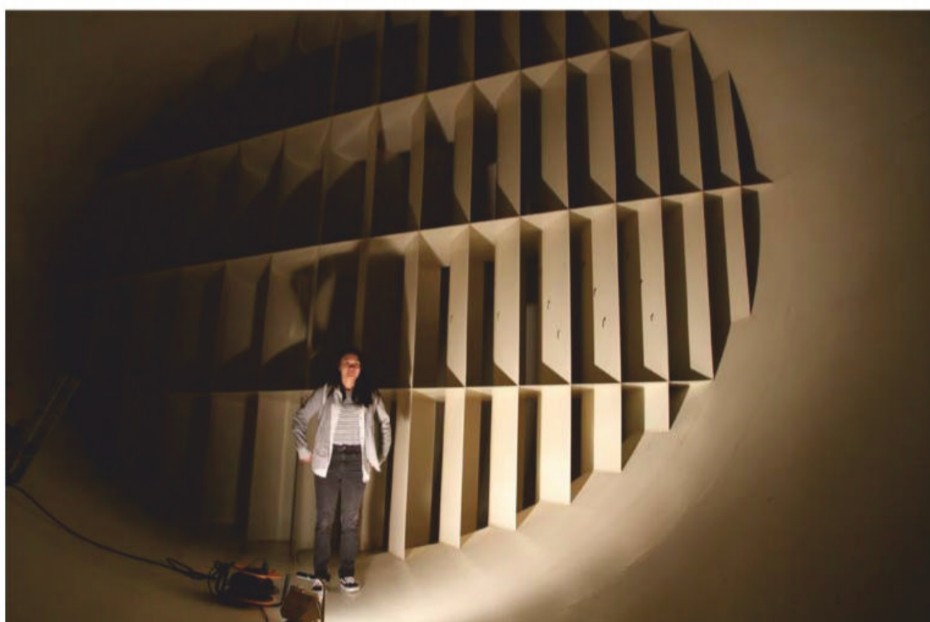
To avoid big losses the tunnel corners are equipped with turning vanes, which are either highly cambered plates or aerofoils
