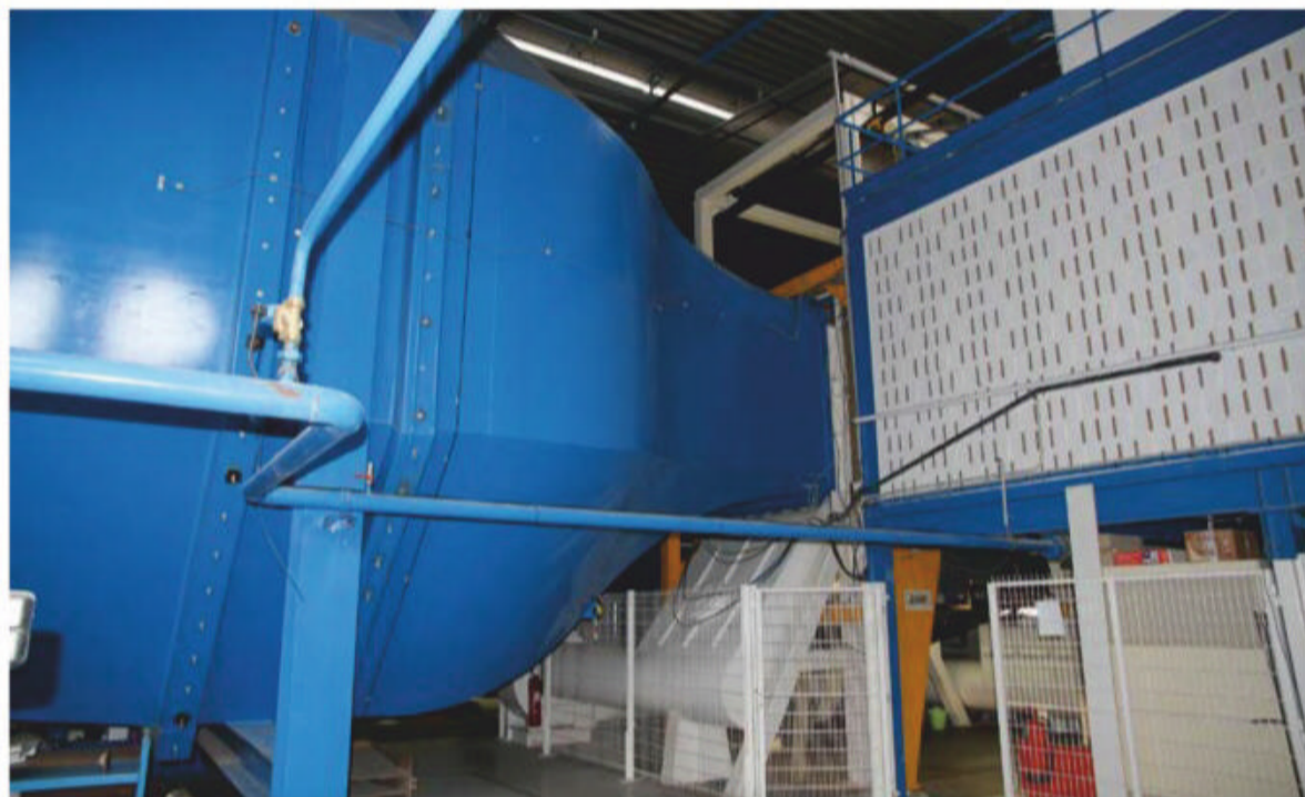
The contraction cone is to accelerate the airflow from the low power-loss speed to the test section speed
