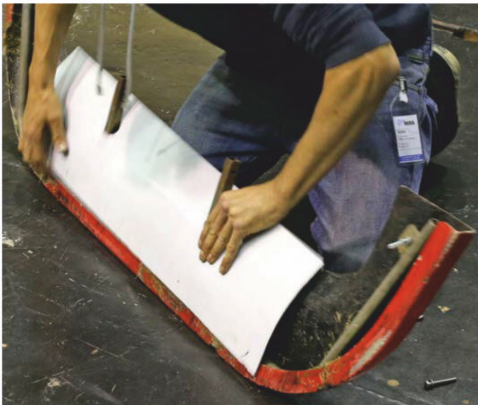
Angled infill panel fitted below the splitter worked as expected, increasing downforce
