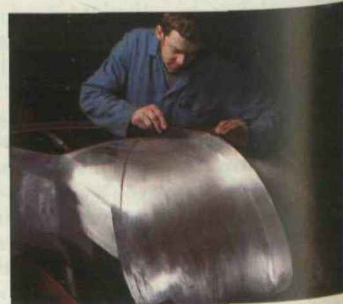
Fine attention to detail given to contouring tail of Alfa Romeo 8C/2.3.
