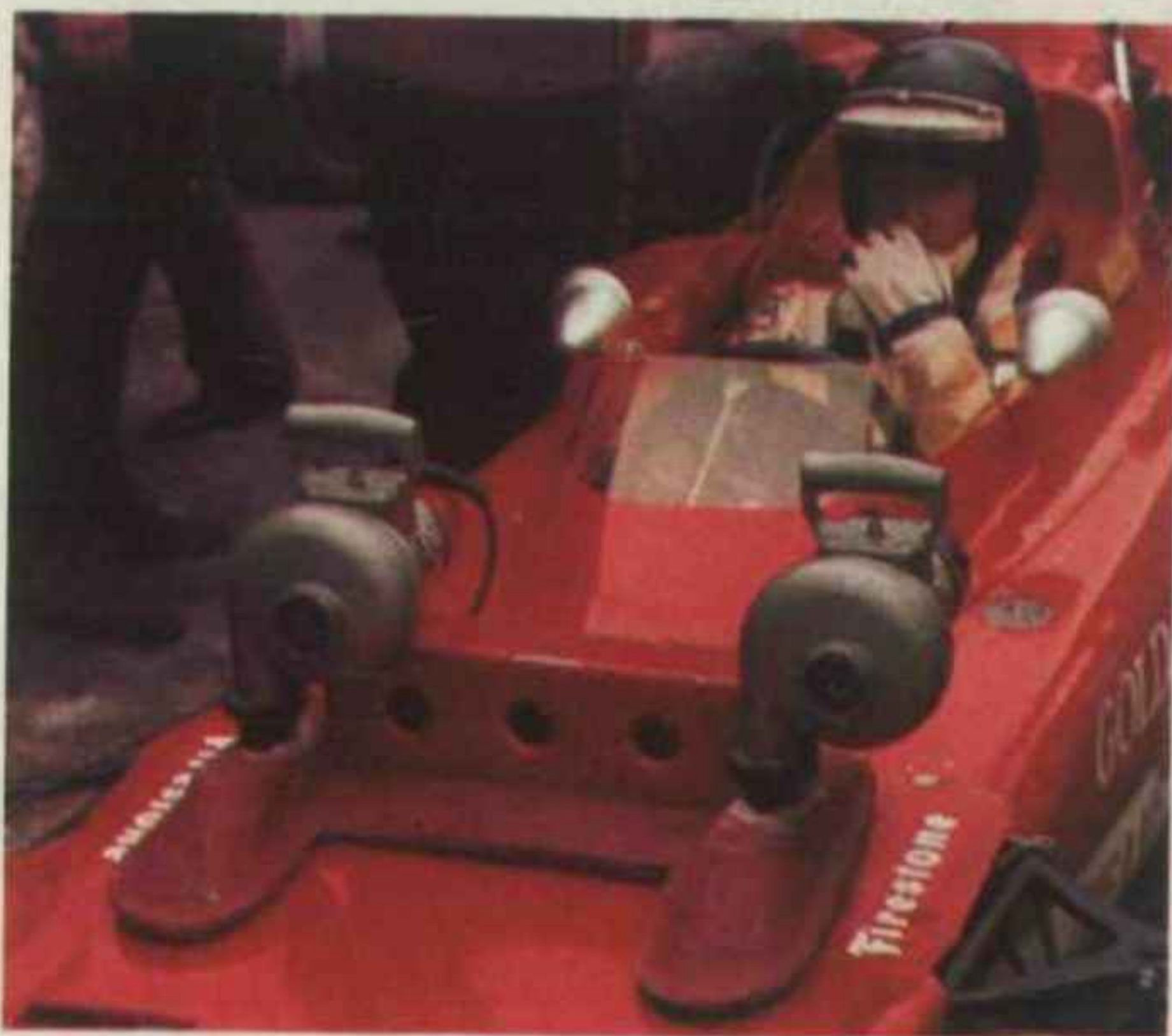
Lotus 72's inboard brakes brought snags. Coolers on Rindt's 72 (left) helped stop brake spacers melting
