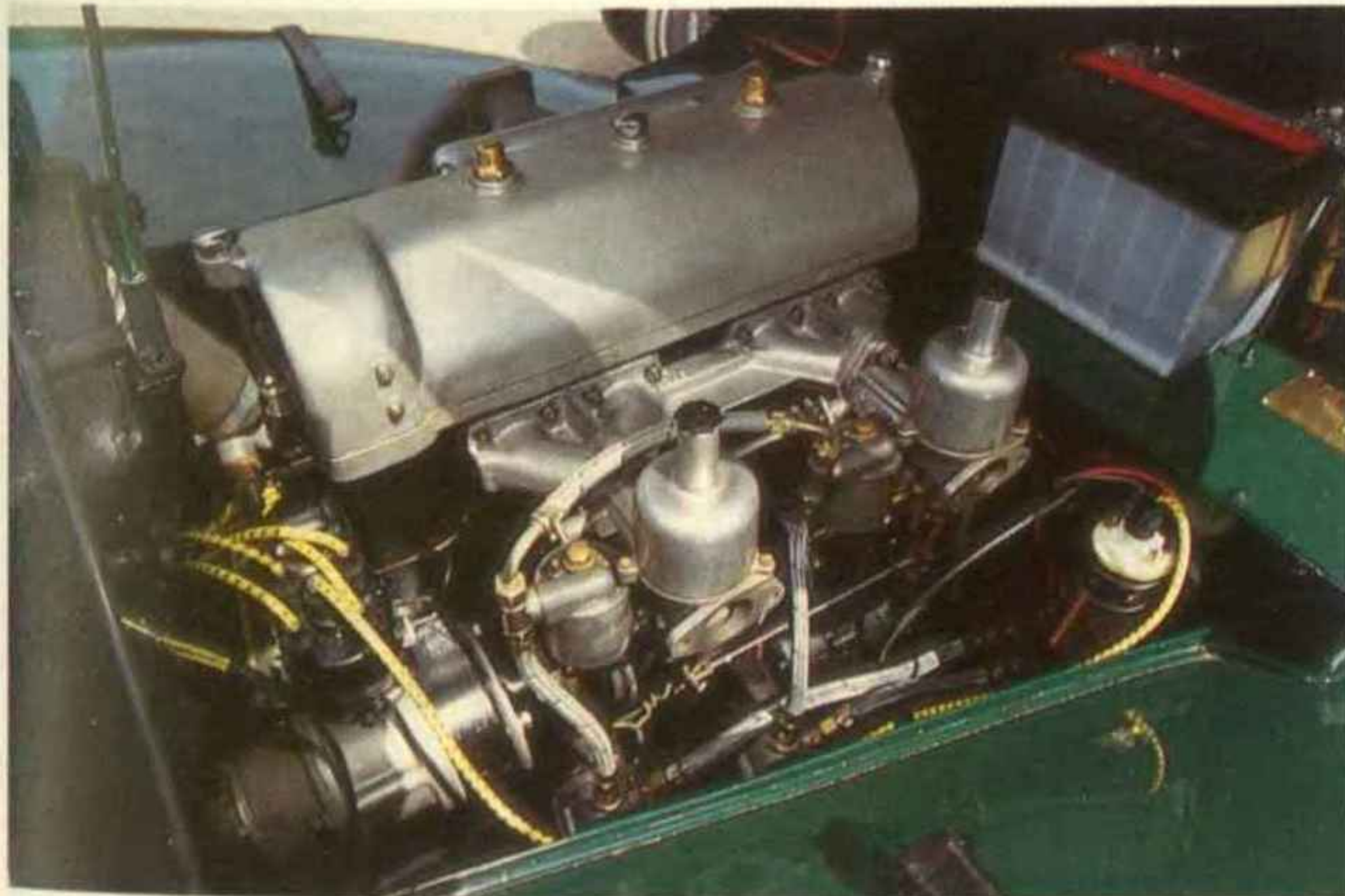
One-piece bonnet lifts up to show dry sump 2-litre ohc Bertelli motor. Works claimed 105bhp which, says Bell, is a bit optimistic
