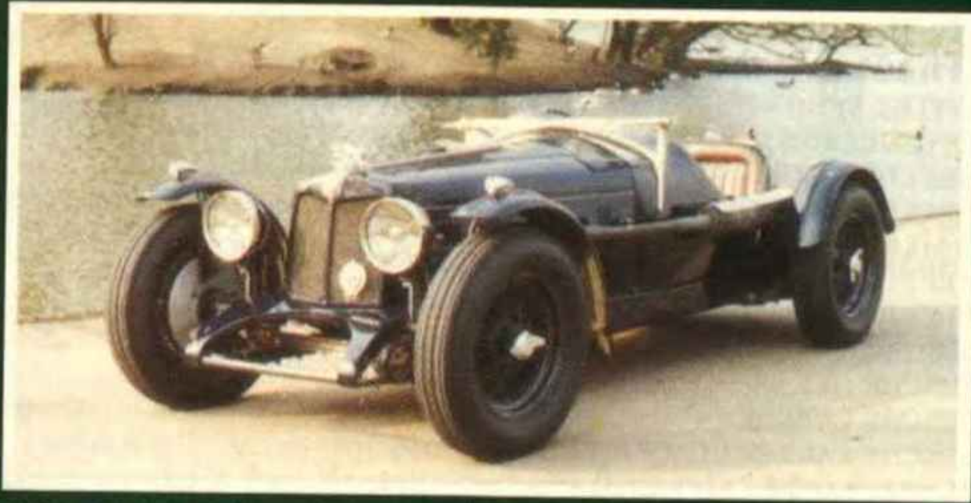
1934 MG KN SPECIAL. 1600cc six cylinder engine with Volumex supercharger, Carello rods, Mahle pistons, special one piece steel long crank, etc. Body by Rod jolly. Superbly engineered and very fast.
