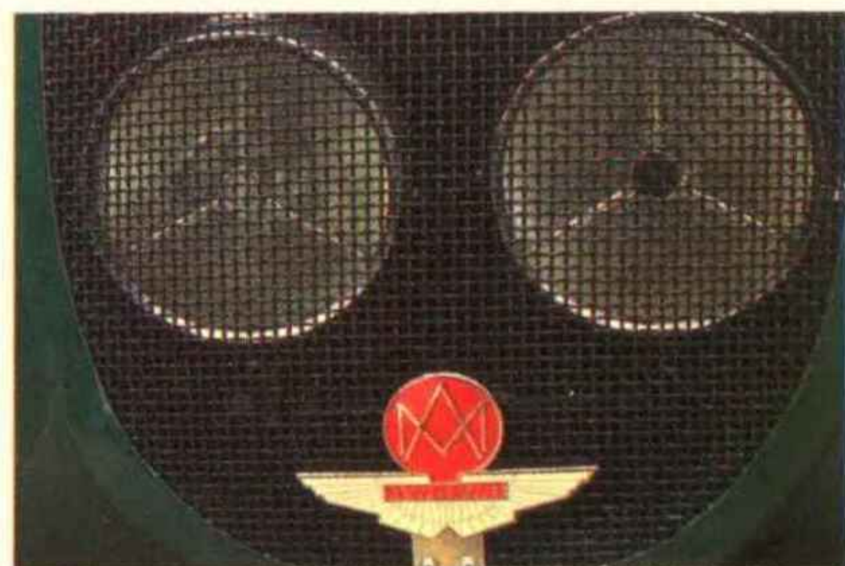
Andy Bell of Ecurie Bertelli behind the Aston's elaborate fascia, above. Headlamps mounted inside grille cut drag. Aero-body reunited with chassis after seven years apart. Nose and grille were only new panels
