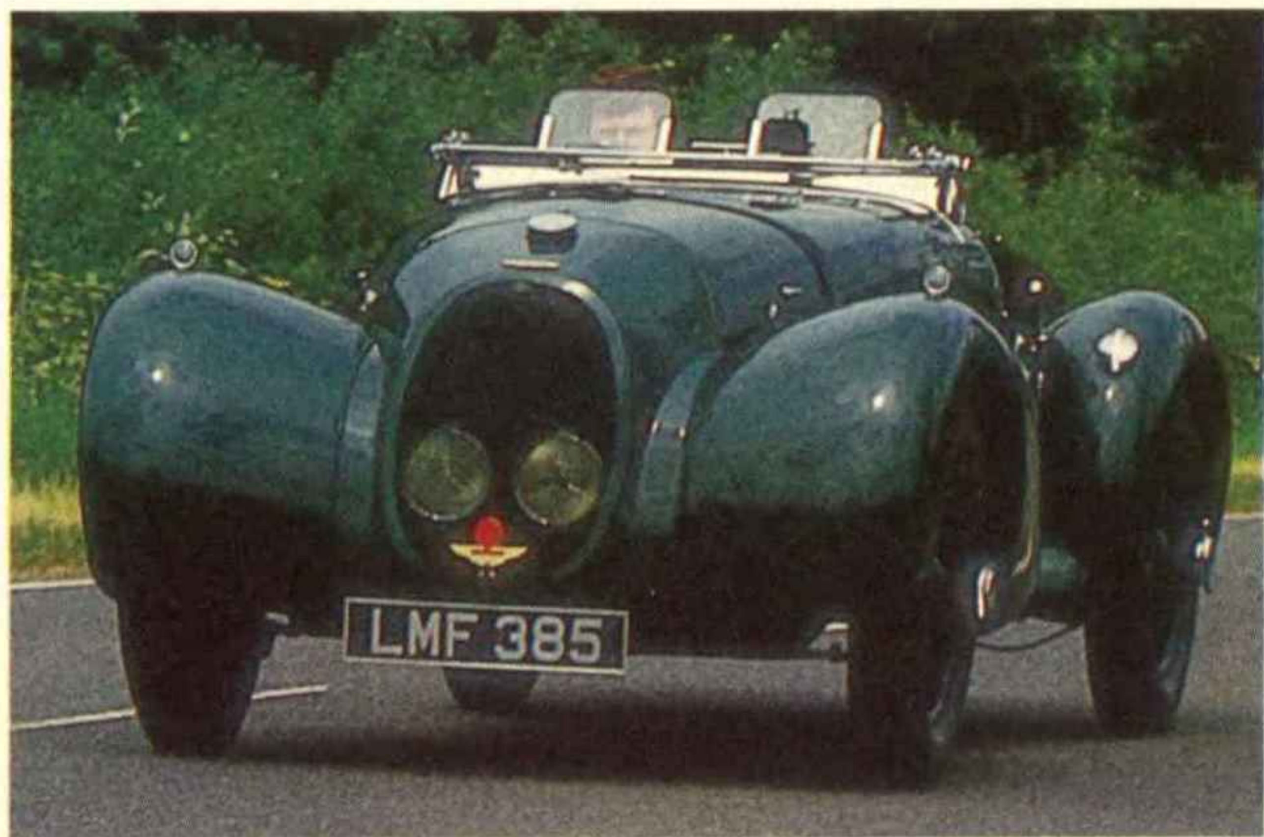
Andy Bell of Ecurie Bertelli behind the Aston's elaborate fascia, above. Headlamps mounted inside grille cut drag. Aero-body reunited with chassis after seven years apart. Nose and grille were only new panels
