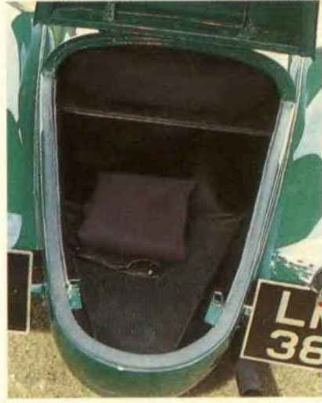
Instruments, along with many small detail parts, had survived with car. Tail locker offers minimal storage; spare wheel lies behind seats. Teardrop tail profile evident
