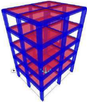
Figure 2.3D view of the Structural model
