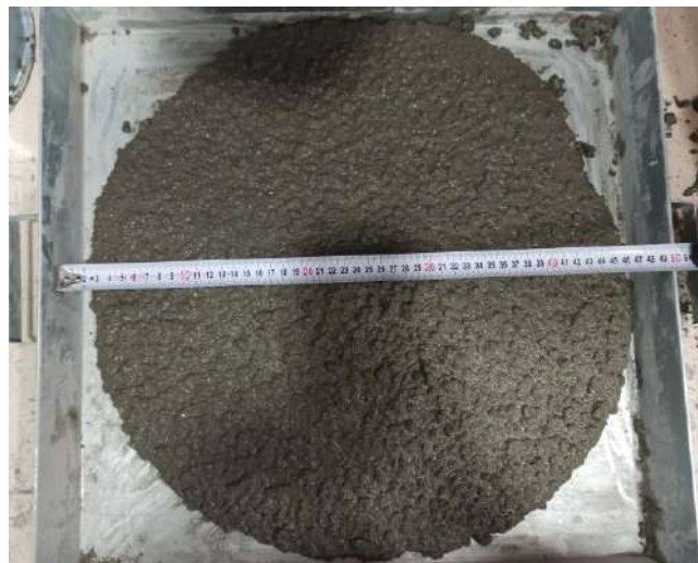
Figure 1. Slump flow measurement of self-compacting concrete
