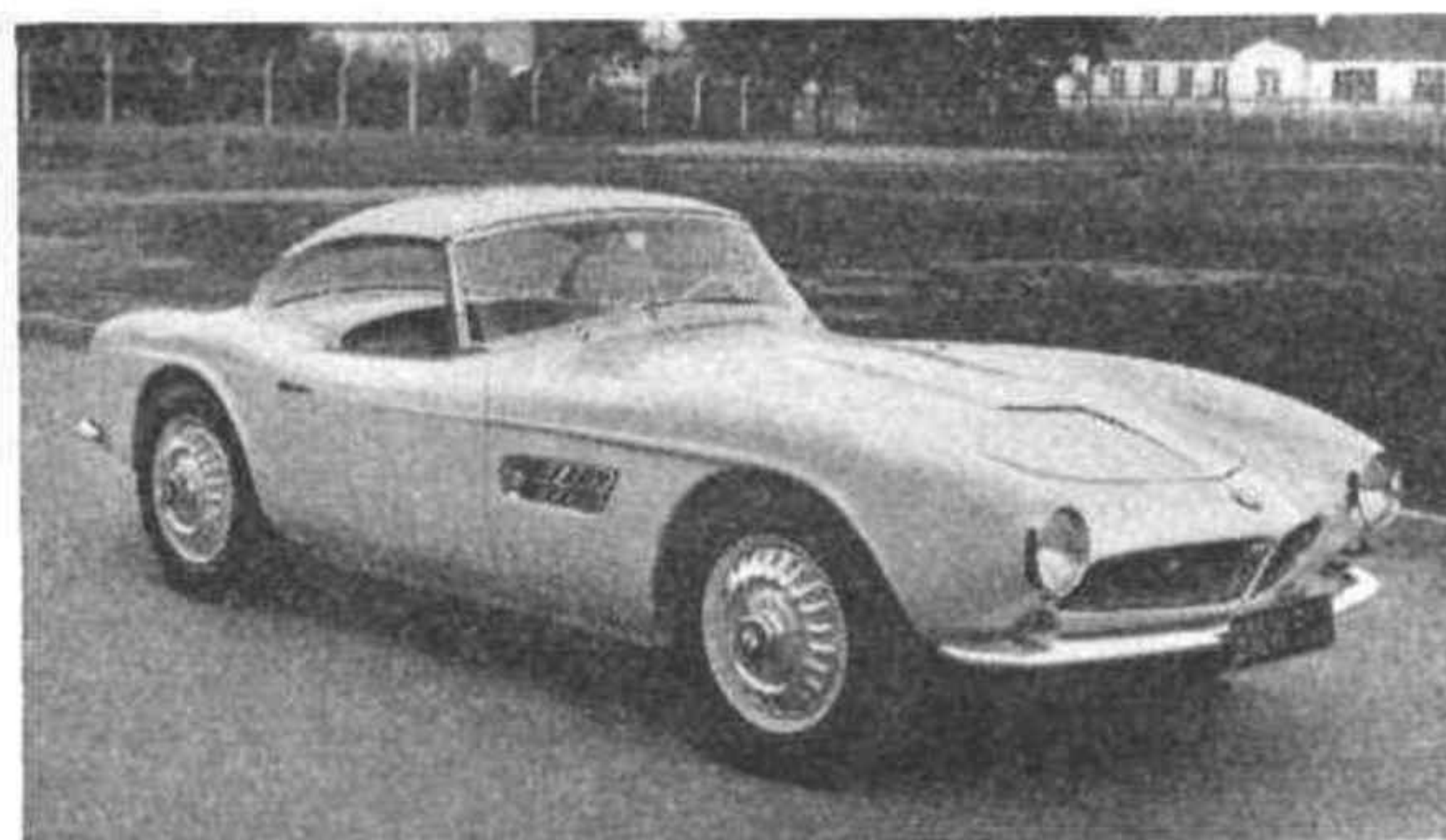
EXCITING NEWCOMER. —The B.M.W. 507 sports-roadster with detachable aluminium hard-top. This car looks better than photographs make out, which is an unusual state of affairs, and in this view it looks very pretty anyway. Fitted with the V8 engine enlarged to 3,168 c.c., with bore and stroke of 82 by 75 mm., it runs to 5,500 r.p.m. and develops peak power of 140 b.h.p. at 4,800 r.p.m. The knock-off splined hubs as shown are an extra, normal five-stud wheels being standard.
