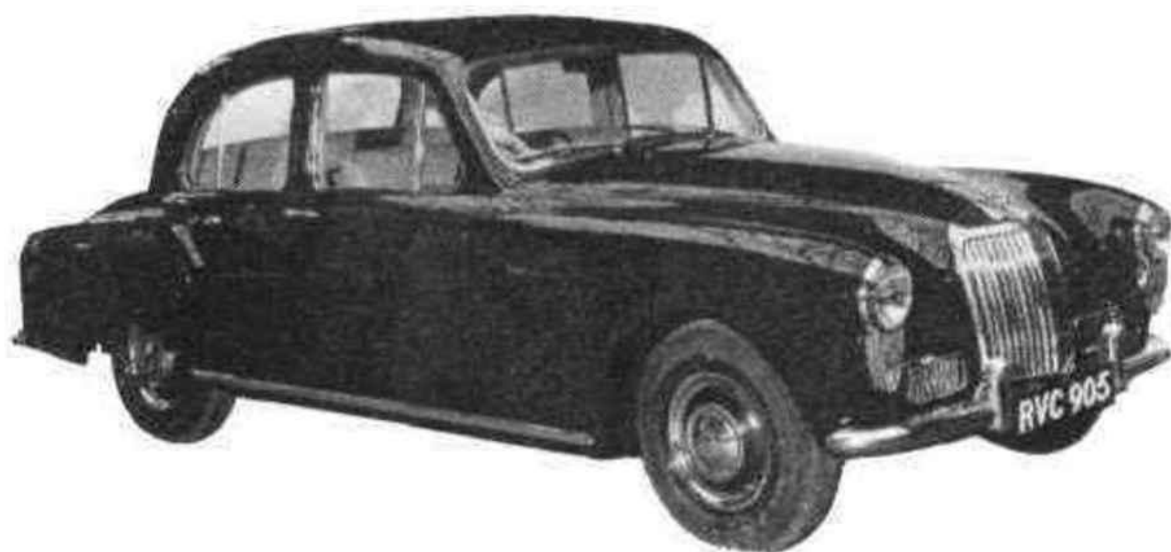
THE HUSH-HUSH 2.3-litre Armstrong-Siddeley Sapphire 234, which with four-cylinder cross-push-rod o.h.v. "square" engine, develops 120 b.h.p. and for which 100 m.p.h. is claimed.
