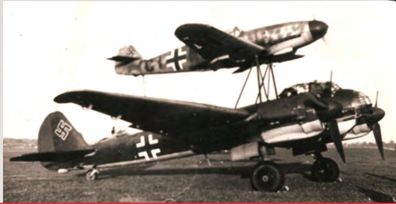
Left The prototype Mistel composite, Bf 109F-4 'Cl+MX', atop a Ju 88A-4 during trials at Ainring, west of Salzburg, early 1944.
