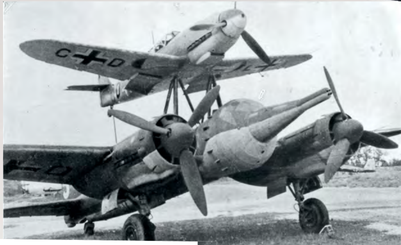
Left An operational Mistel with the Ju 88A-4 element fully modified with the hollow-charge warhead and probe-mounted proximity detonator. The Bf 109F-4 is 10130 'CD+LX'. Both were lost on the night of June 14, 1944.
