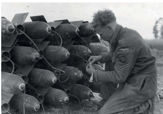
Right: A groundcrew man works on the electrical connections of a stockpile of 60lb RPs. The weapons were almost certainly destined for use on Typhoons. RAF (AHB)/© UK MoD Crown Copyright 2014
