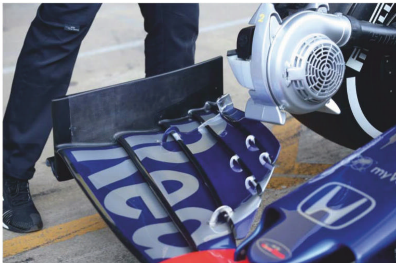
To try to eliminate outwash very simple end-plates have been mandated for the front wing. Toro Rosso STR14 is pictured
