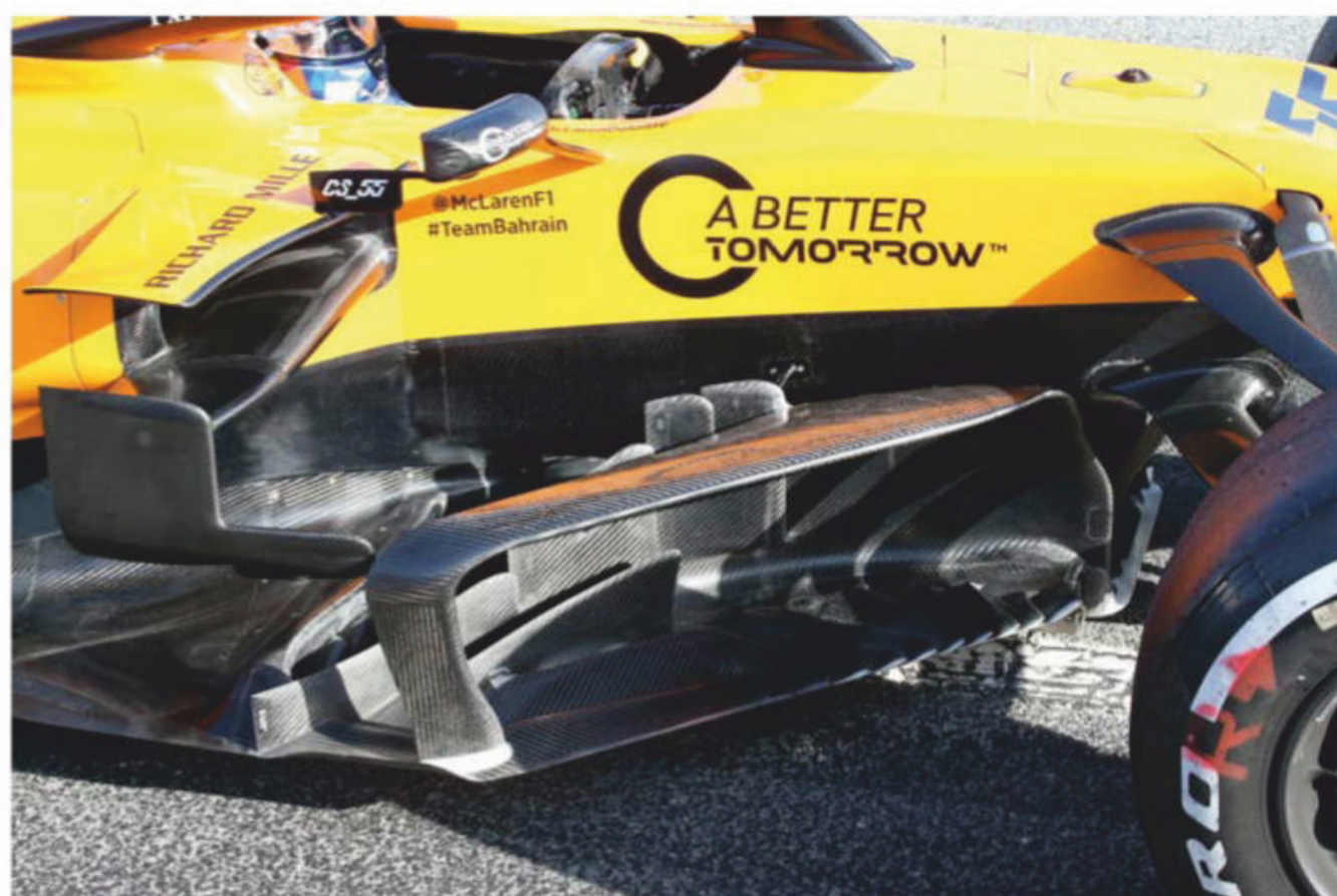
The bargeboards on the McLaren MCL34 feature a bridge section. This remains a prime area for development in Formula 1
