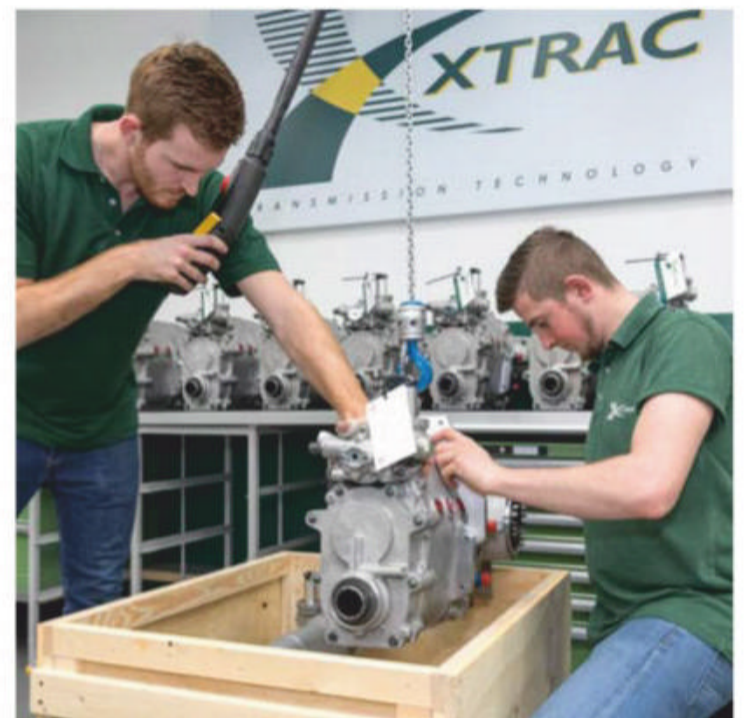
For this season Supercars has switched to a new Xtrac 6-speed gearbox which has been specifically designed for the category
