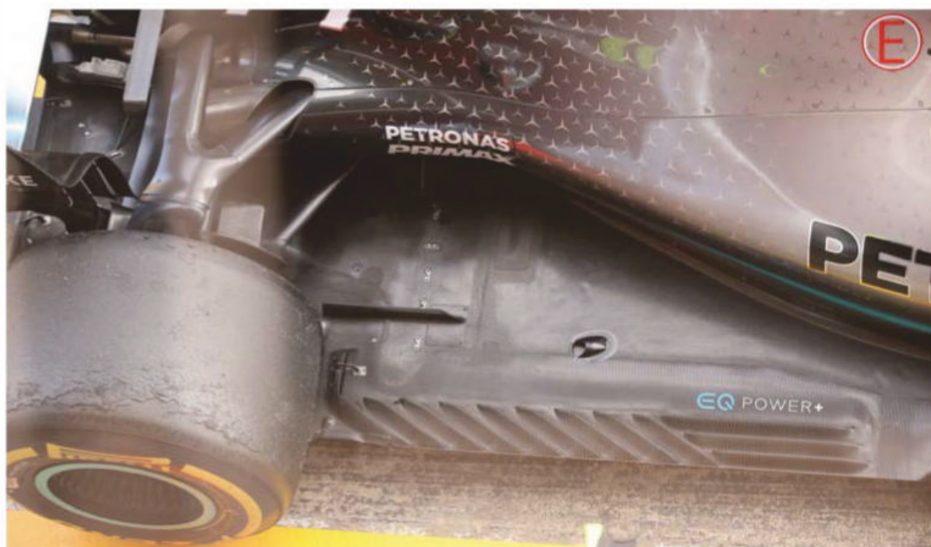
Rear tyre sensors are generally mounted in a blister on the floor. Thermal imagers will often be found in this location too
