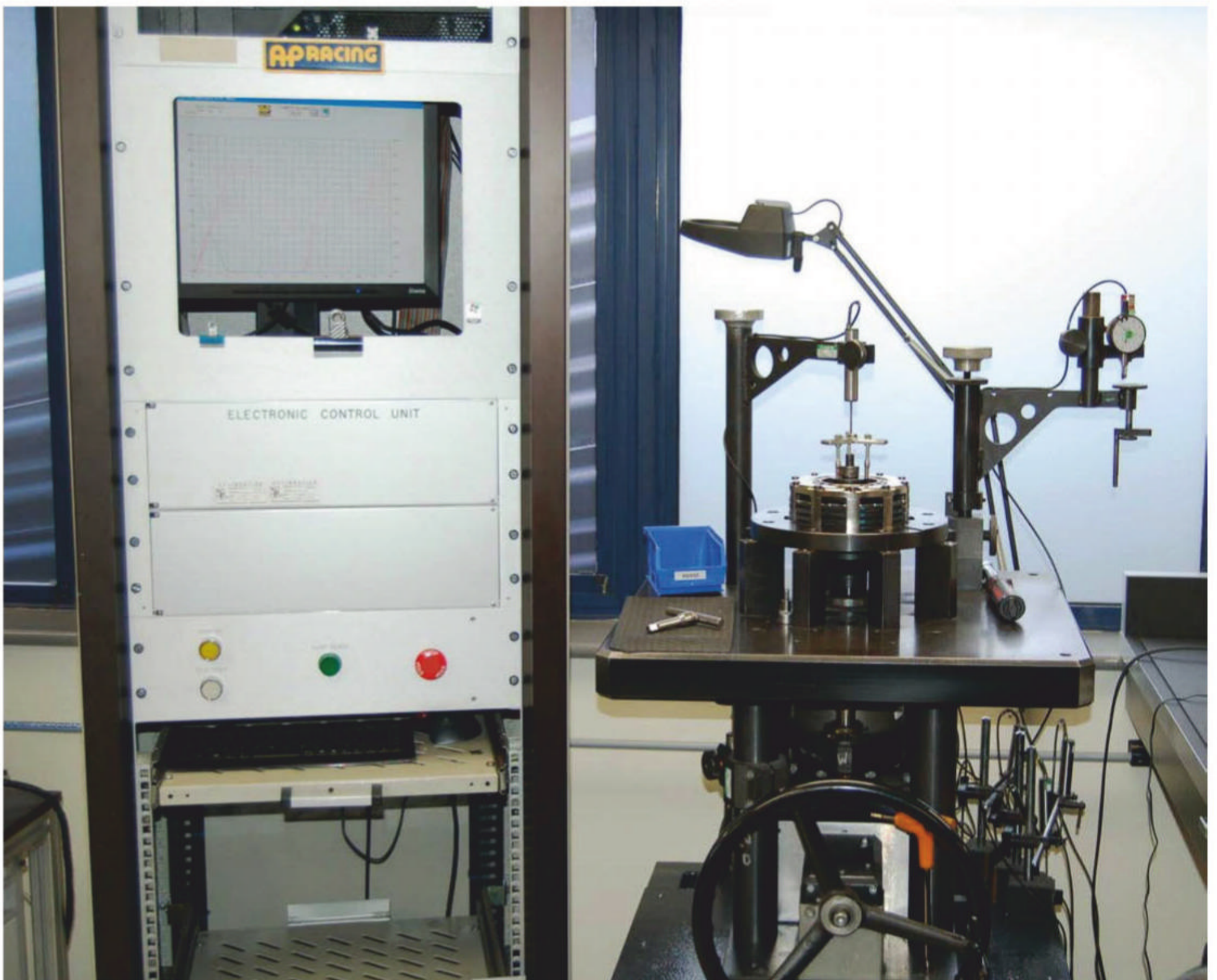
Clutch control: Each and every carbon clutch that AP Racing has manufactured for motorsport applications has been tested on a rig to gather data on its particular characteristics
