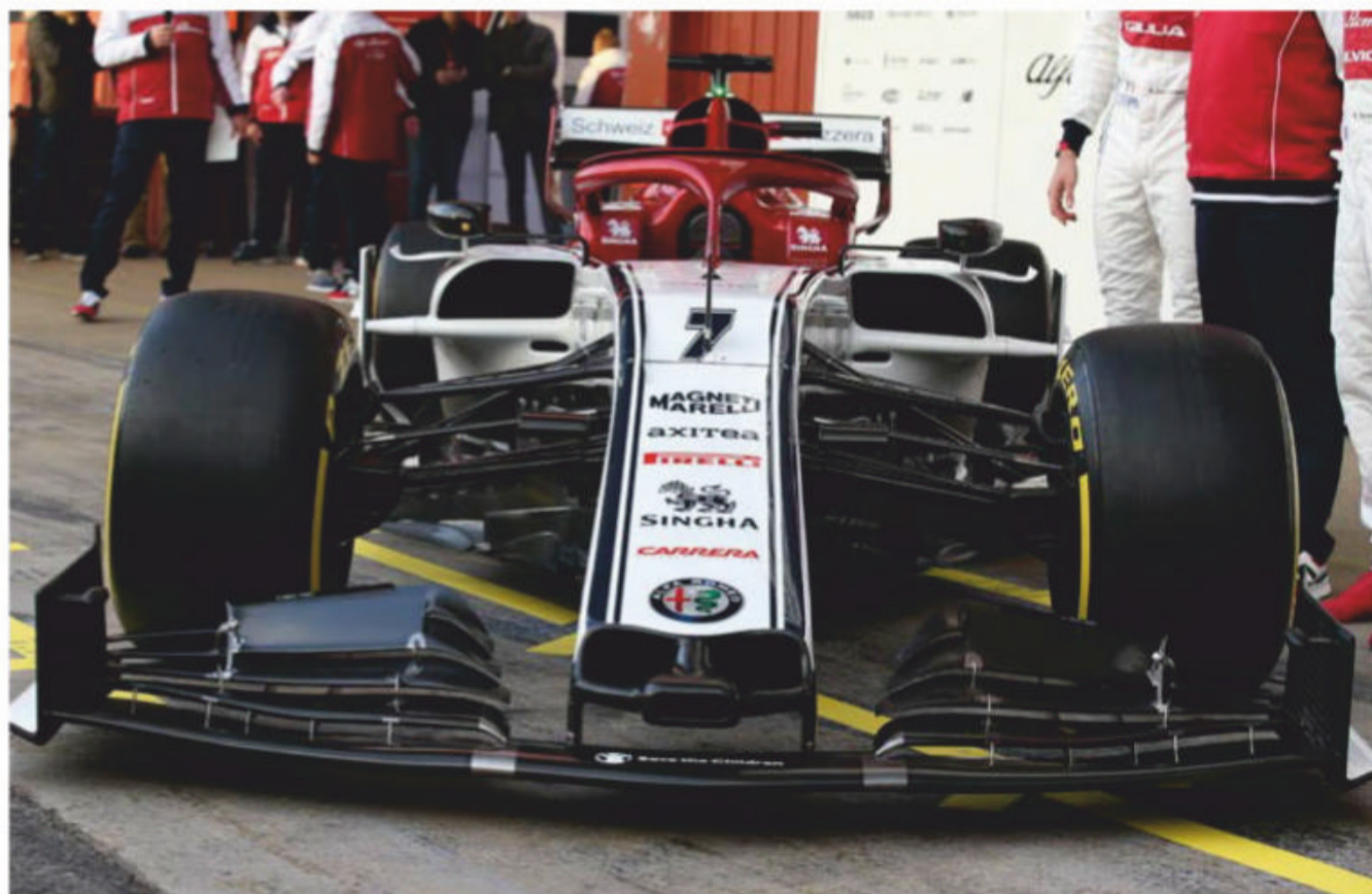
The front wing on the Alfa seems to be designed to encourage outwash, with flatter upper elements on the outer portions
