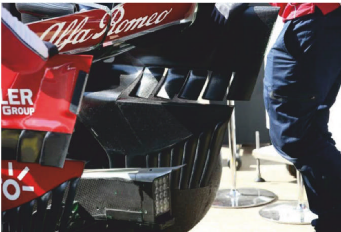
Rear wing end-plates are getting quite complex with some designs featuring distinct upper and lower sections
