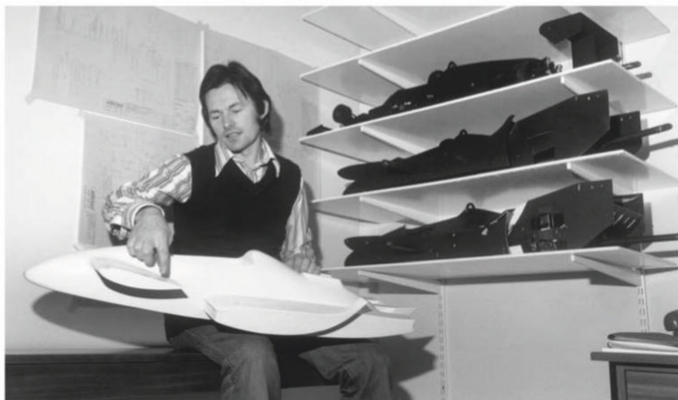
Tony Southgate in late 1979, pointing to the flap at the rear of the 'wing section' that was used to adjust aero balance
