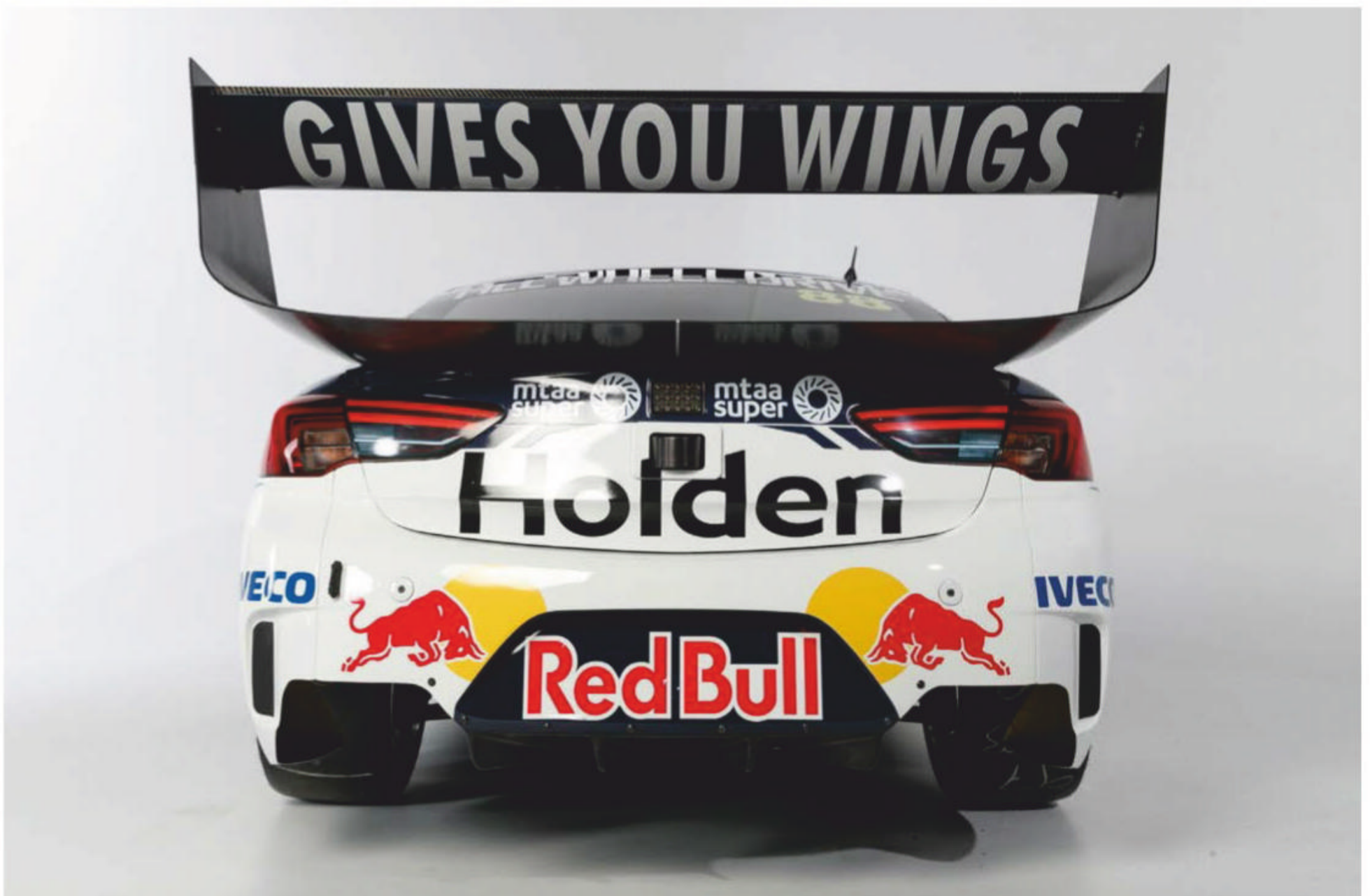
Being sponsored by Red Bull really does give you wings. Changing the rear wing angle is one of the very few things the teams can do to tune aero performance after homologation
