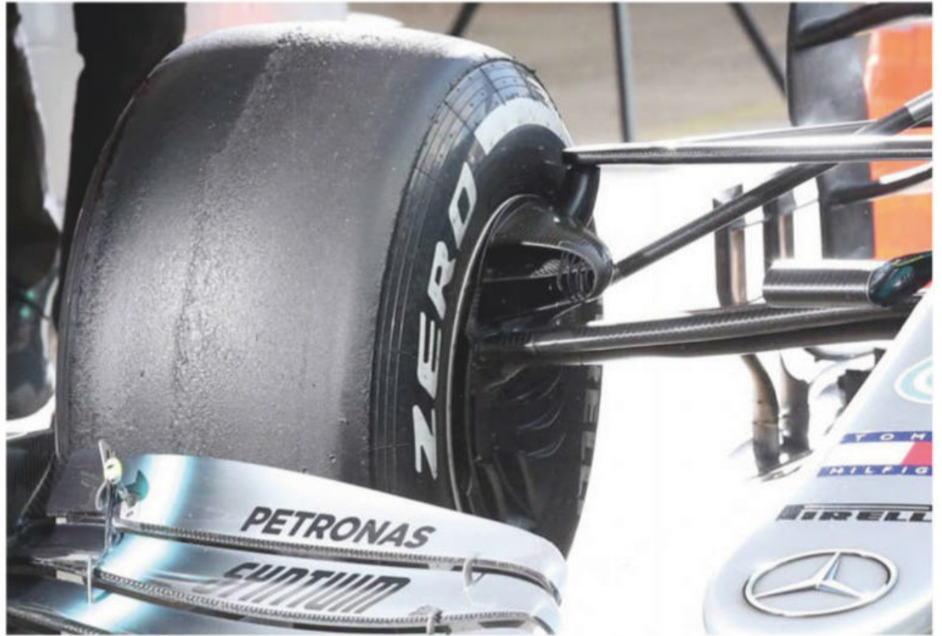
The Mercedes W10 sports a highly developed front brake duct with a cluster of small aero elements sitting inside the wheel
