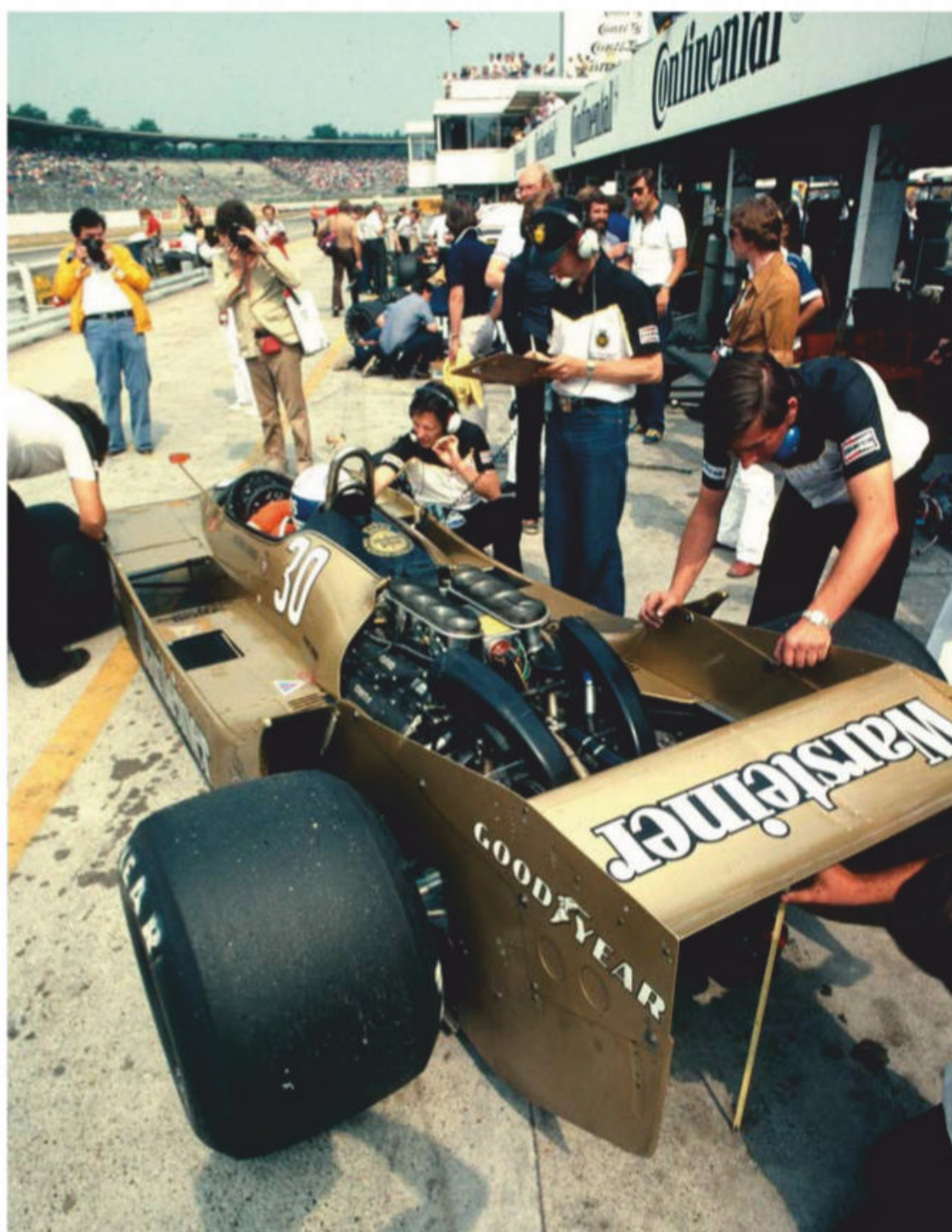
The A2 was originally going to have an almost fully enclosed engine, but overheating issues scuppered that plan
