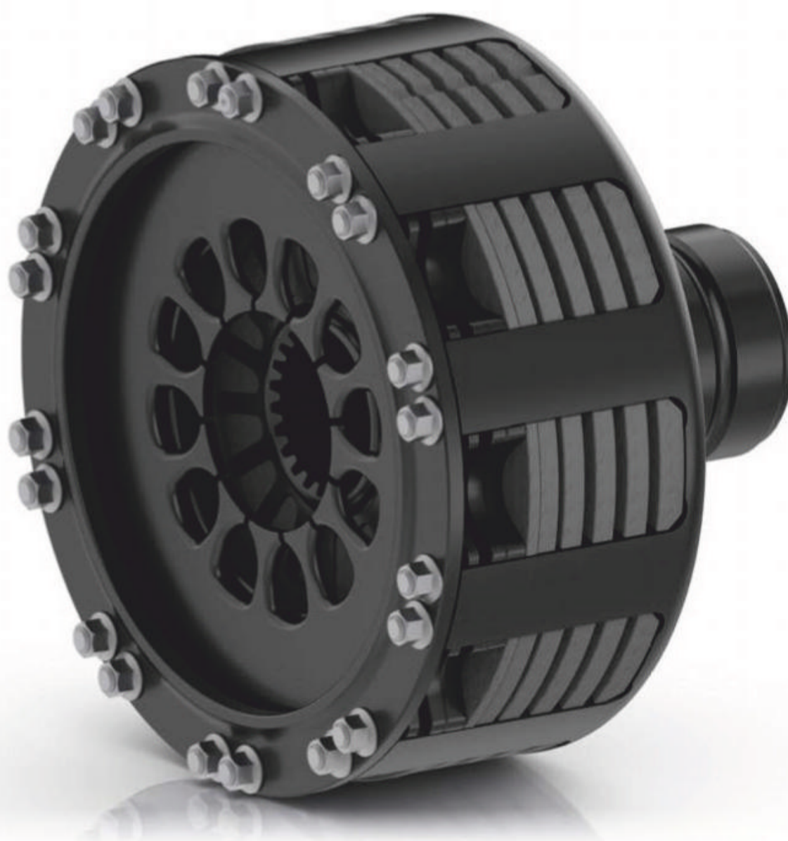
In F1 the switch to V6 turbos in 2014 increased engine torque, so to cope with this higher torque capacity clutches went from three-plate to four- or five-plate. The four-plate F1 clutch is shown above and in exploded view below
