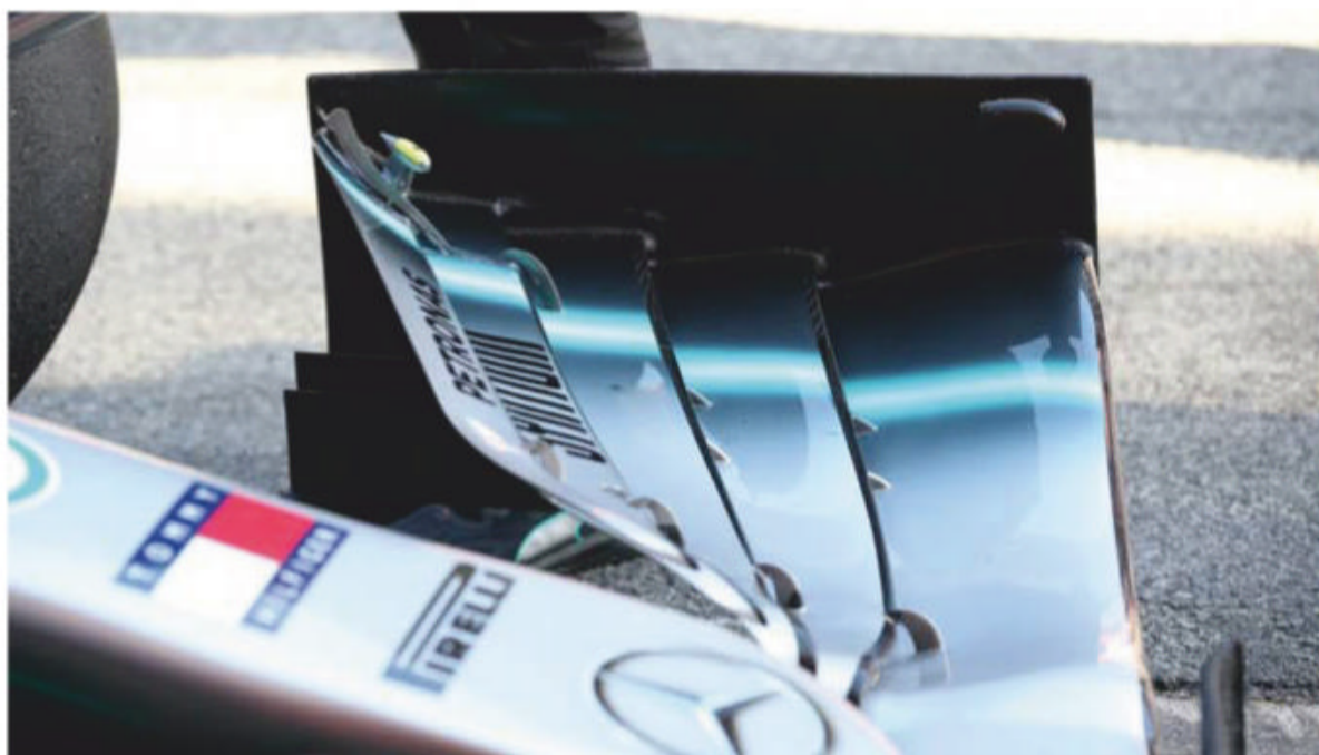
Mercedes has a multi-channel IR sensor mounted on the front wing end-plate, as close as possible to the tyre
