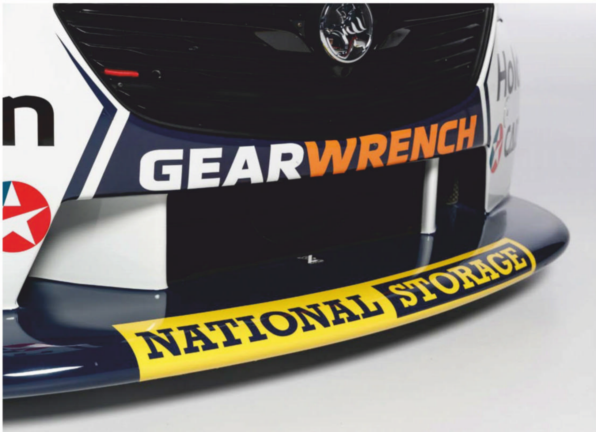
Air for cooling the brakes can be provided via a controlled opening in the front of the racecar. This can only be adjusted, to tune for tracks and the conditions, with blanking plates
