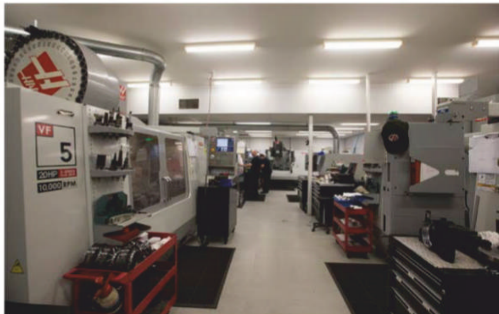
Three CNC mills and two CNC lathes allow Triple Eight to manufacture everything from uprights to engine components in-house
