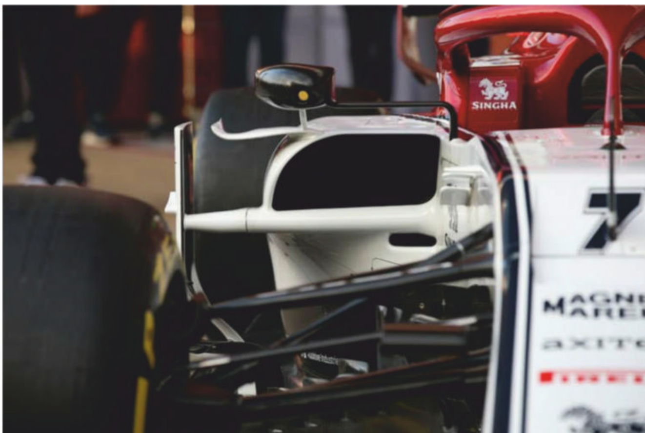
The Alfa Romeo has its tyre sensor mounted in the mirror housing, but this location has caused issues for teams in the past
