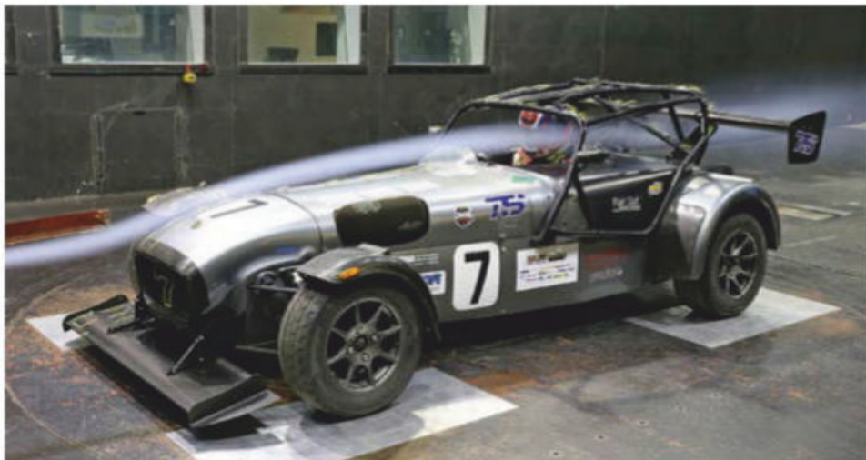
Front and rear single element wings plus wheel arch Gurneys adorn the Caterham R400
