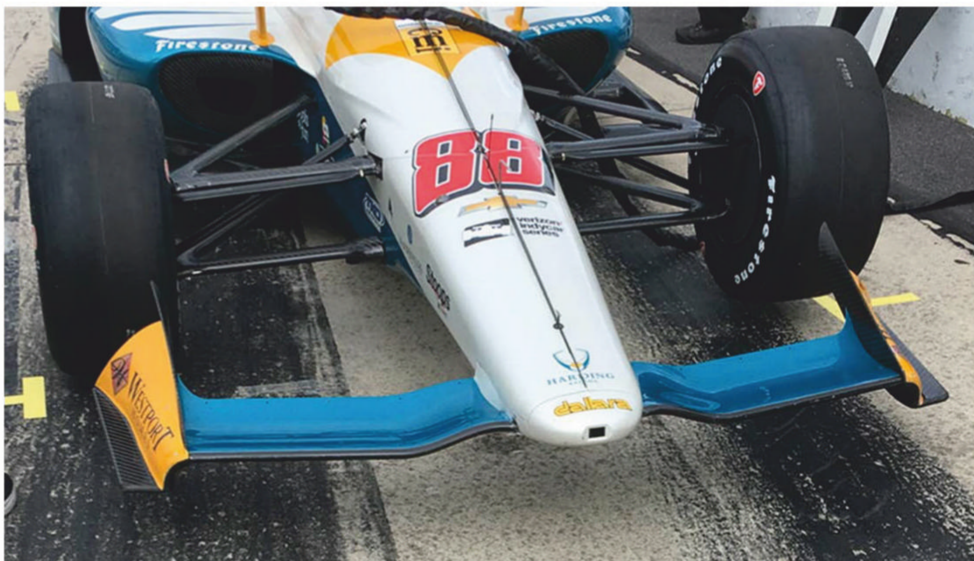
The UAK18 wing was less complex than those on the 2017 aerokits. One effect was that more air reached the floor, which was biased towards the rear, and this led to an imbalance
