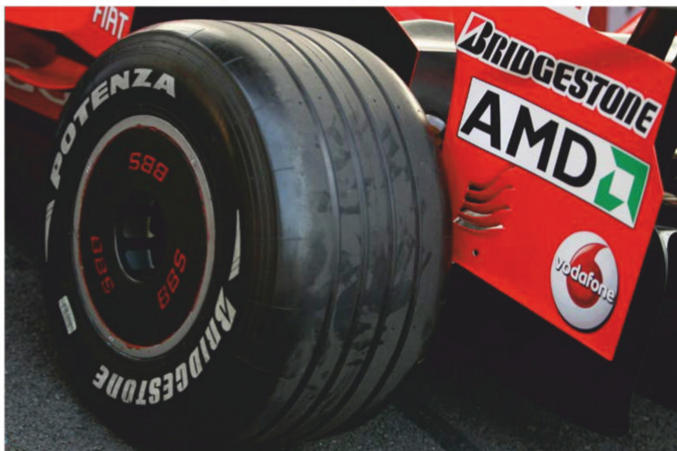
Drag reducing wheel covers, as seen here fitted to the 2006 Ferrari, could be a feature of Formula 1 cars from 2021
