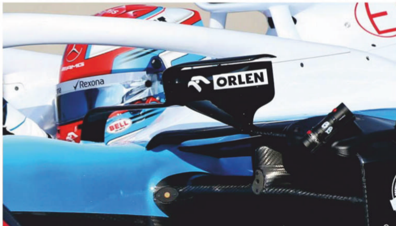
The mirrors on the Williams FW42 perhaps give a hint of the direction in which the aero development in this area will go
