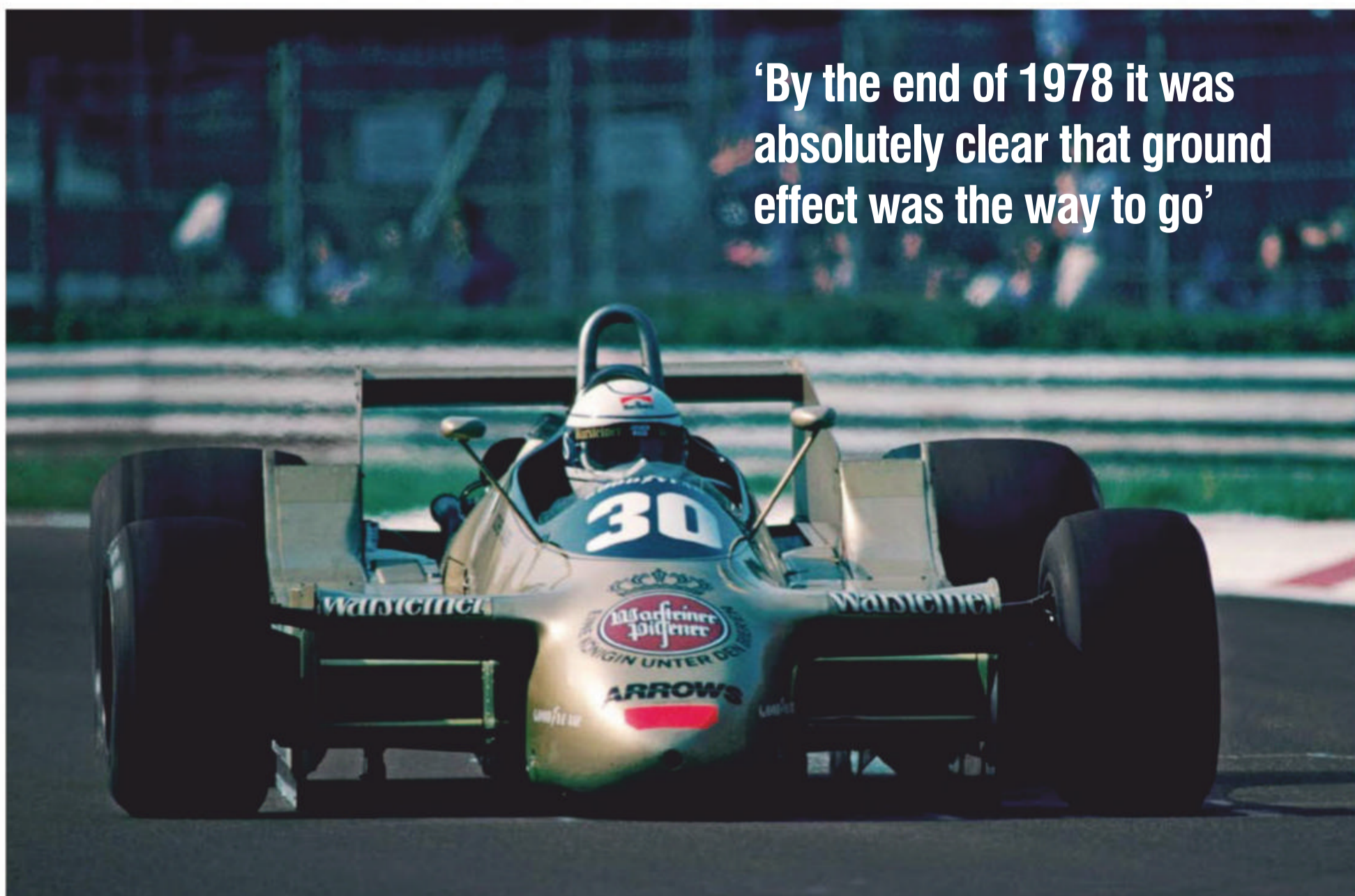
The A2 was designed to run without a rear wing yet one was fitted by the time of its second race; but this was more to do with driver confidence than producing downforce
