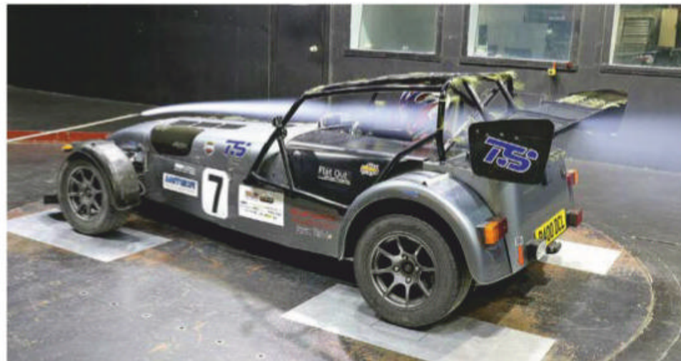
The rear wing proved to be effective even though it was mounted behind the roll cage
