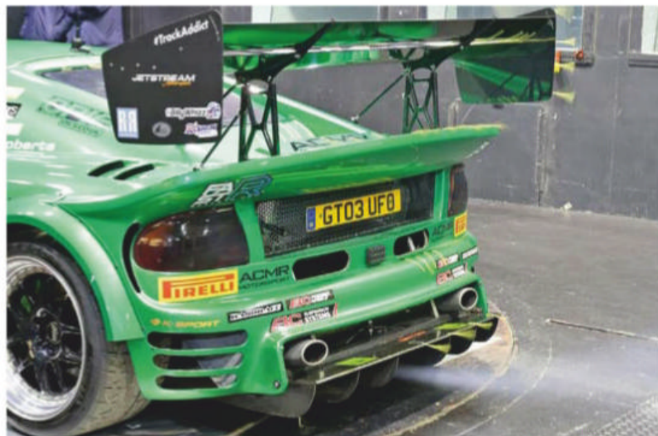
The Noble's wing, spoiler and diffuser all interacted to help generate high downforce
