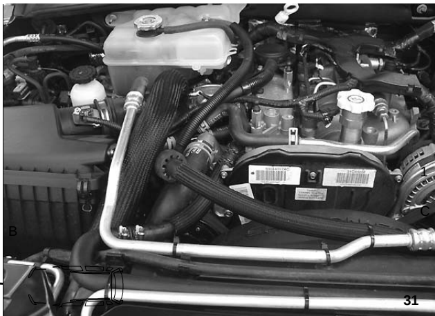
B Water hose "B"1 Hose clip Ø 27mm C Water hose "C"
