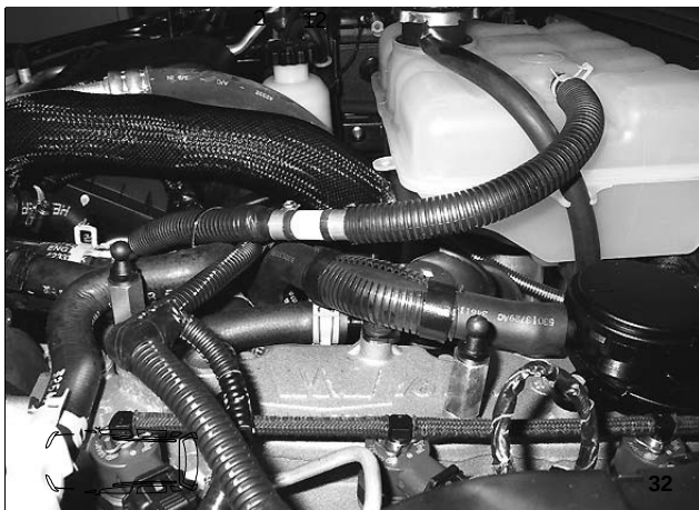
Check valve 2 x 12 acc. Figure in line to the reservoir einsetzen. Achtung: Pay attention to flow of the check-valve!
