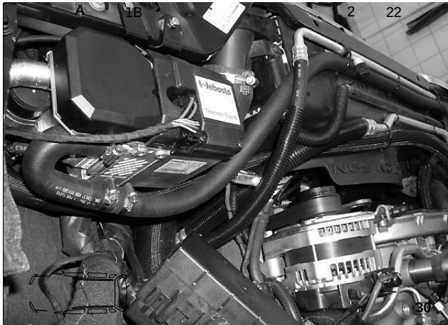
A Molded hose "A"1 hose clamp B Water hose "B"2 Cable ties (3x)
