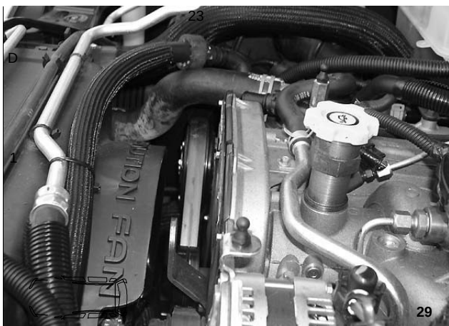
1 cable ties2 Rubber profile black3 Hose clip Ø 27mmD Water hose "D"
