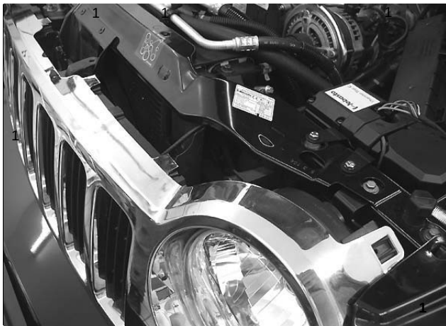
1 Clips of the grille mounting
