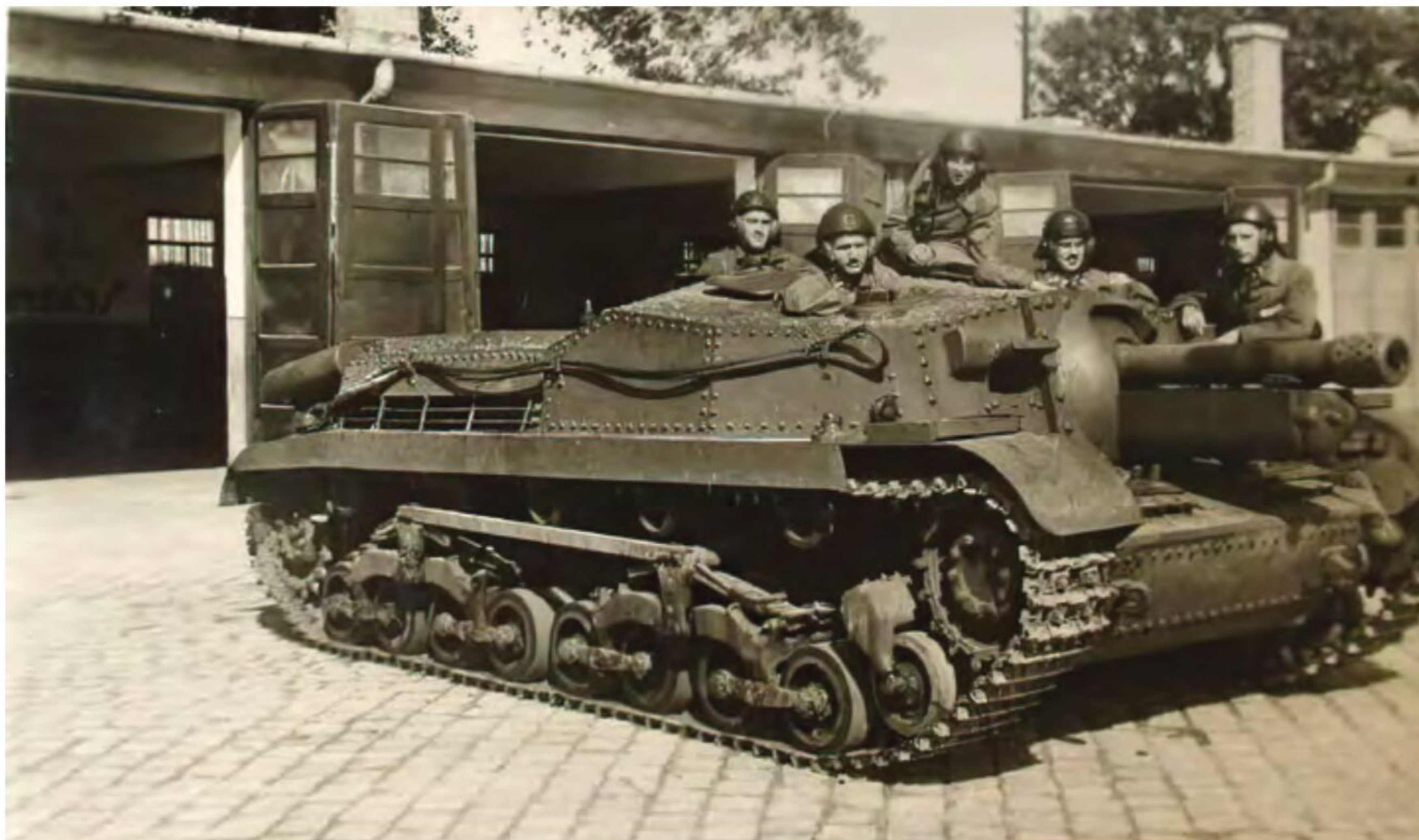
BELOW RIGHT: Assault artillerymen with their early production 40/43M Zrínyi assault howitzer with the Turán-style driver slot, at the yard of the Assault Artillery Training Cadre at Hajmáskér in summer of 1944 DEÁK
