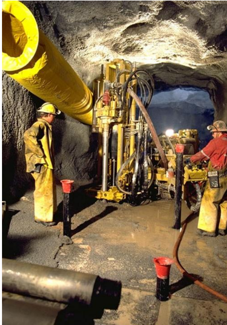
Photo 1 Typical Blasthole Stopping Drill Crosscut at Eagle Point
