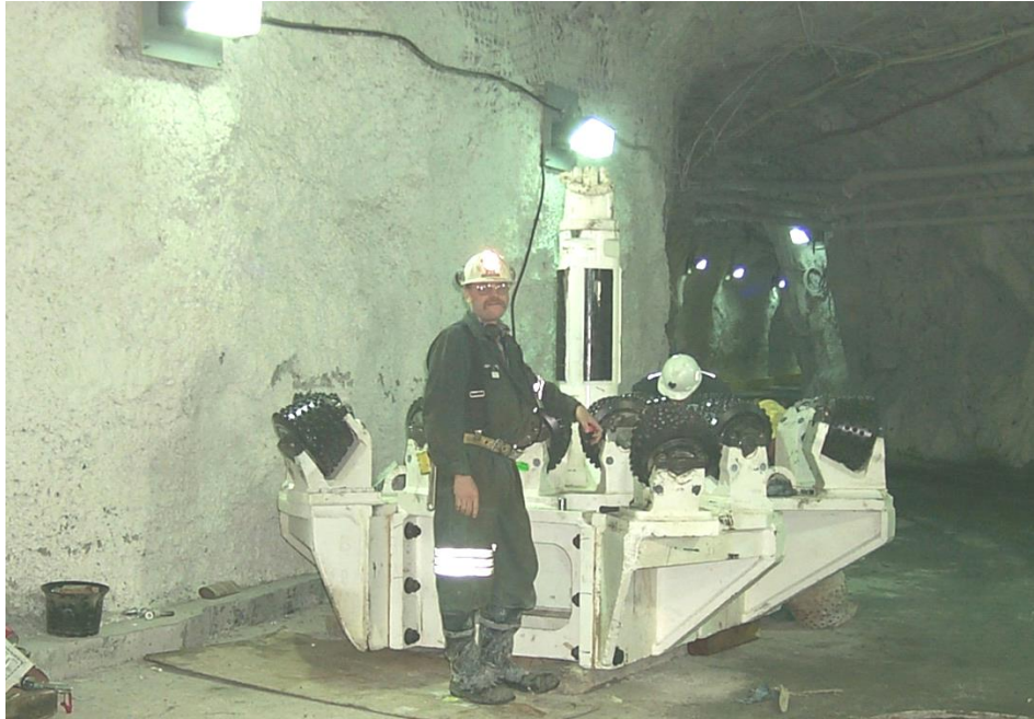
Photo 3 3.0 m Diameter Reamer for Production Raiseboring
