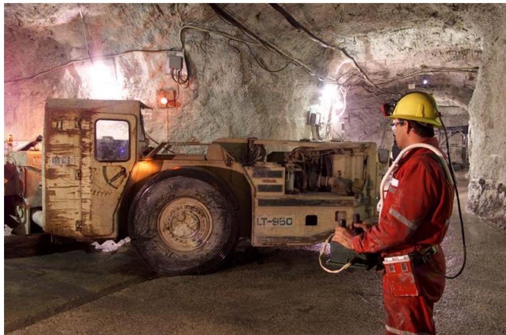
Photo 5 Retrieving the Remote Controlled LHD from the Ore Collection Chute
