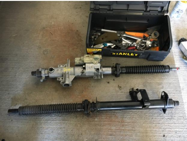
As you can see in the picture above, the original black jacket tube has a welded two-bolt flange. The adjustable one has a detachable one (lacking here).
