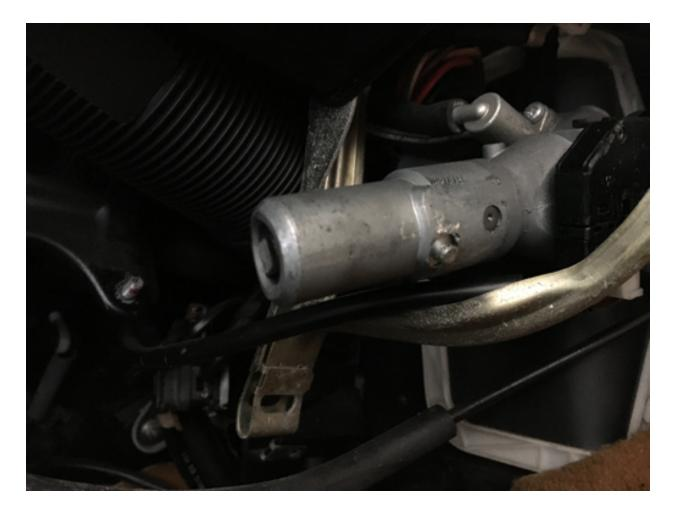
12. At this point, jack the driver side of your car up, secure on jack stand and go under. Locate the 6mm allen bolt connecting the lower steering column to the steering box coupler. Spray with penetrating oil and remove. DO NOT STRIP IT. 13. Now you should be able to pull the jacket tube out with minimal force. Be careful not to bend it.
