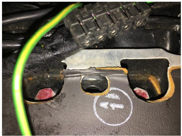
11. Put the key in ignition and turn to position 1. Place a screwdriver in the security hole and push button therein. It can be hidden behind a metal clamp (use 10mm socket to loosen it and move). You should be able to wiggle the whole ignition off.
