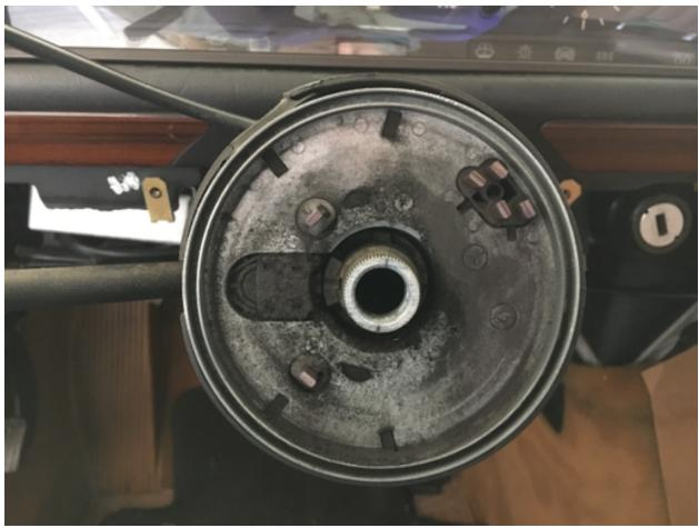
8. Unscrew 3 small Philips screws, remove the plate. Disconnect its cable near the cruise amplifier (red connectors).
