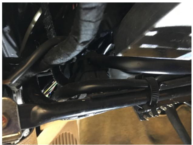
10. Undo 2 10mm nuts holding the jacket tube (steering column) to the shaft. At this point, you have to remove the instrument cluster completely and use a deep 10mm socket to remove two bolts holding the steering column to the upper frame.
