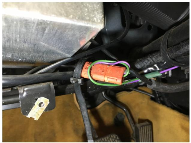
9. Undo 3 bigger Philips screws. Follow the cables and disconnect connectors. Pull the whole plastic cover with signal controls out.
