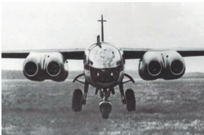
The Ar 234 V8 was powered by four BMW 003s, but problems were encountered with this prototype configuration. VIA CHRIS GOSS
