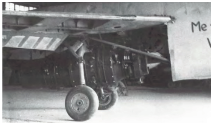
A mock-up of Heinkel's HeS 011 engine fitted to the first, unflown, Messerschmitt P1101 fighter prototype. NASM
