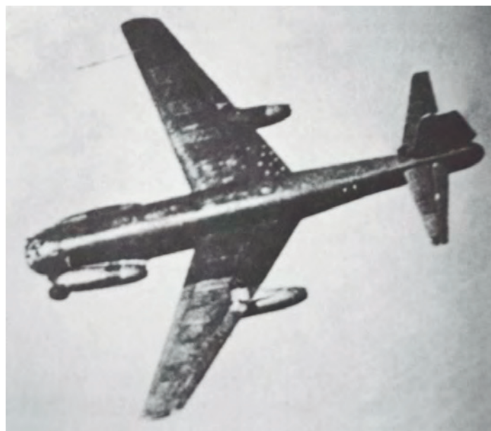
Another use of the Jumo 004, in B-1 guise, was in the Junkers Ju 287 experimental jet bomber, here in four-jet Ju 287 V1 form. The V2 and V3 versions upped the powerplant count to six. KEY COLLECTION
