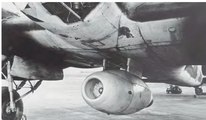
A very rare image of an HeS 8A unit mounted below a Heinkel He 111 for testing in 1941. EN ARCHIVE
