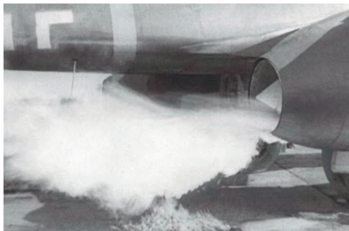
Caused by unburnt fuel in the exhaust, a fiery start-up for a III./EJG 2 Me 262. VIA CHRIS GOSS
