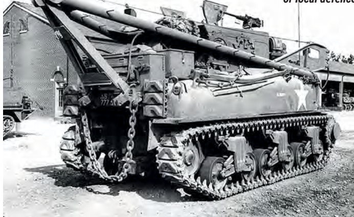
Rear view of World War Two M32 fully stowed and with heavy tow chain. The 0.50 machine gun is fitted for anti-aircraft or local defence
