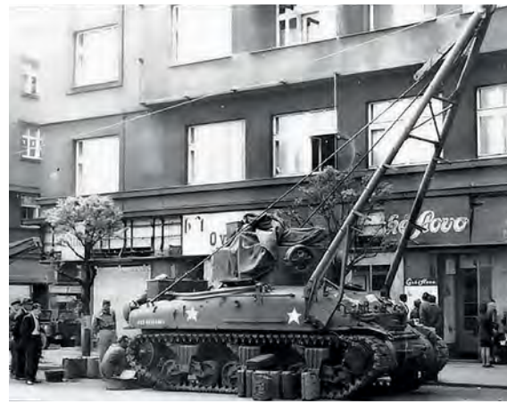
RIGHT (FROM TOP): M32B1A1 near Humhung during the Korean War. Note HVSS suspension. WIKIMEDIA COMMONS; World War Two photo showing an M32 with extended crane ready to start lifting. The Jerrycans at the side show signs of recent refuelling; The M32 was based on the chassis of a Sherman tank. WIKIMEDIA COMMONS; ARV crew cook supper in front of their vehicle while local children wait for a share. Note 81mm mortar in ready position
