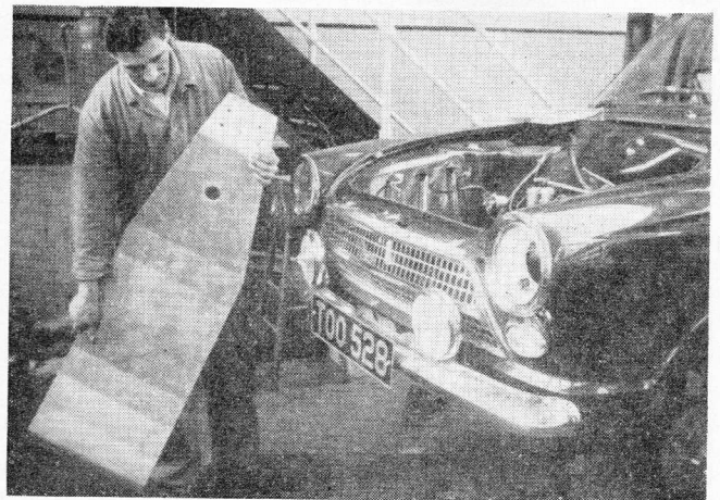
FORD: Jack Welsh (left) lowers a Cosworth 92 b.h.p. 1,200 c.c. engine into an Anglia. On the right, Norman Masters prepares to fit a \frac{1}{4} in. dural sump guard to a Cortina.
