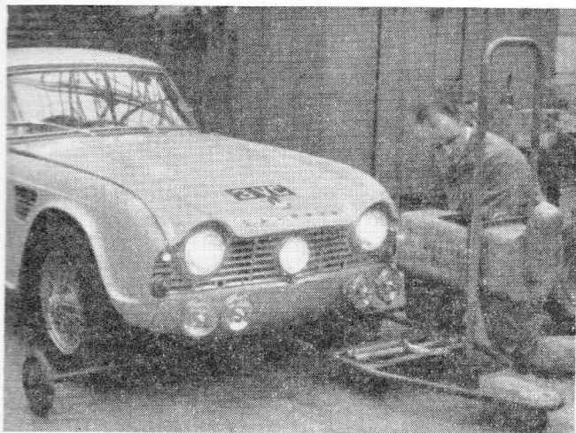
TRIUMPH: Les Harris (left) checks the lamps on a TR4. In the centre of the grille is a long-range pass-lamp which goes out automatically when the sealed beam headlights on each side of it (top row!) are dipped. The four lamps at the bottom are all fog-lamps which can be used by themselves, or in pairs in conjunction with headlights. RIGHT: Note the cooling louvres on the TR4 receiving attention from Ray Anderson and Roger Sykes.
